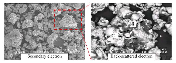
*Figure 1.* SEM micrographs of particles from a binder-treated mix made of ATOMET 1001, 2% Ni, 0.85% graphite and 0.75% wax+binder. C represents either graphite or lubricant.
