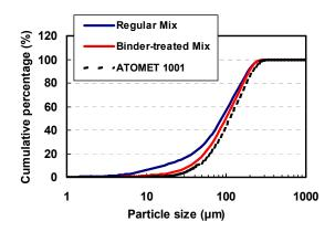
*Figure 2.* Particle size distribution of regular and binder-treated FLOMET mixes (laser diffractometer).
