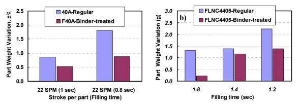
*Figure 5.* Part weight variation for tests carried out under more difficult filling conditions (fill height/wall thickness = 8.2). a) Suction fill b) Gravity fill
