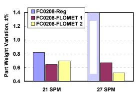
*Figure 6.* Part weight variation obtained during production of drive nuts at two compaction rates. \* Regular mix was not run at 27 SPM.
