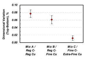
*Figure 7.* Dimensional variation between the top and the bottom of rings made of FLN4-4405 mixes with 4%Ni. 2.6%Cu and 0.5%C.
