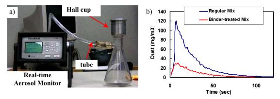
*Figure 3.* Quantity of dust (particles  $< 10 \ \mu$ m) created by a regular and a binder-treated F0008 mixes when powders flow in a recipient. a) Experimental assembly b) Results.
