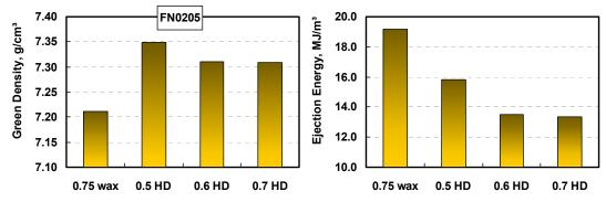
*Figure 10.* Performance of a new lubricant-binder system under development for high density applications. a) Green density b) Ejection energy (FN0205 mixes pressed at 60°C and 840 Mpa)
