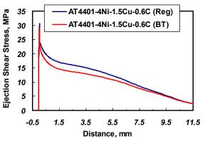
*Figure 9.* Ejection curves for FLN4-4405-1.5% Cu mixes with 0.65% EBS wax. AT4401 refers to ATOMET 4401 (0.85%Mo steel powder).
