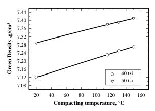
**Figure 1.** Effect of compacting temperature and pressure on green density of specimens pressed with a mix of ATOMET 1001+0.6% grap.+2.5% Ni, using die
