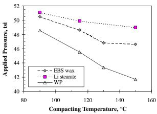
**Figure 12.** Effect of compacting temperature and lubricant type on the applied pressure needed to reach a density of  $7.2 \text{ g/cm}^3$ , ref (Mix: FN-0205 + 0.6% Lub).
