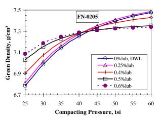
Figure 14. Compressibility curves of warm pressing FN-0205 mixes with different level of lubricant. (Compacting temperature : 130°C)
