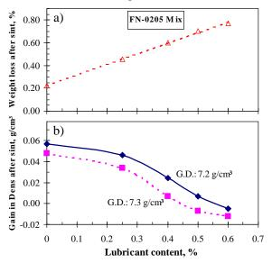
**Figure 6.** Effect of the lubricant content on a) weight loss after sintering and, b) gain in density after sintering (FN-0205 mixes).
