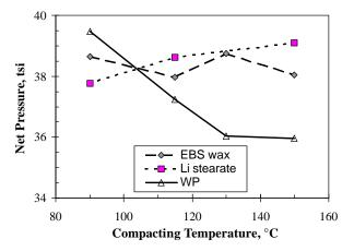
**Figure 10.** Influence of the lubricant type and the compacting temperature on the compactability of FN-0205 mixes, ref. . (pressed to 7.25 g/cm<sup>3</sup> IN-Die, 0.6%Lub)
