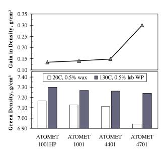
Figure 4. Effect of compacting temperature and lubricant type on green density and the gain in density of various steel powders (Steel + 0.6% Grap. + 0.5% Lub, pressed at 45 tsi)
