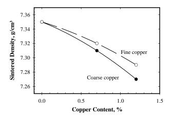
**Figure 8.** Effect of copper content on the sintered density of TRS specimens pressed at 130°C and 45 tsi (ATOMET 4401+3.5% Ni+0.3% C+Cu+0.5% Lub; pressed to 7.35 g/cm<sup>3</sup>).
