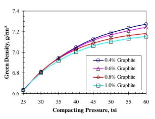
**Figure 7.** Effect of the graphite content on the compressibility at room temperature of mixes made of ATOMET 4401+ 1%Cu + C + 0.75% Zn St
