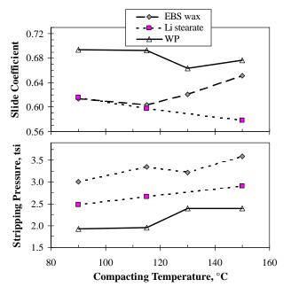
**Figure 11.** Effect of compacting temperature and lubricant type on the lubrication at die walls during compaction and ejection, ref (Mix: FN-0205 + 0.6% Lub, In-Die Density : 7.25 g/cm<sup>3</sup>).
