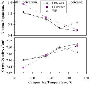
Figure 2. Effect of compacting temperature on the volume expansion at ejection and green density for specimens pressed to 7.25 g/cm<sup>3</sup> IN-Die.
