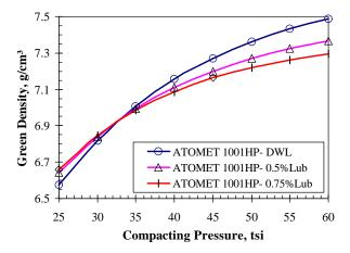
Figure 5. Effect of lubricant content on the compressibility of ATOMET 1001HP at room temperature.
