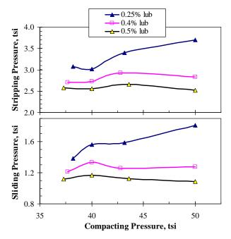
**Figure 17.** Influence of the compacting pressure and lubricant content on the ejection of FN-0205 mixes pressed at 130°C.
