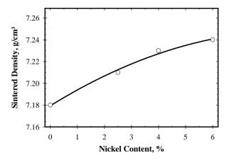
**Figure 9.** Effect of nickel concentration on the sintered density of TRS specimens pressed at 520 MPa and 130°C (ATOMET 4401+0.2% C+Ni+0.55% Lub; pressed to 7.20 g/cm<sup>3</sup>).
