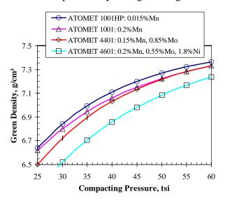
Figure 3. Compressibility curves of steel powders having various concentration of pre-alloyed elements at room temperature (0.5% Lub)
