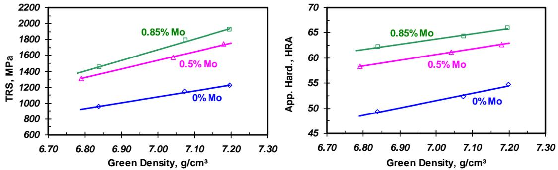
Figure 6. Effect of green density on sintered properties (fast cooling rate + tempered).
