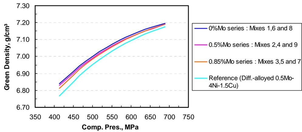
Figure 2. Compressibility curves for mixes regrouped by level of pre-alloyed Mo.
