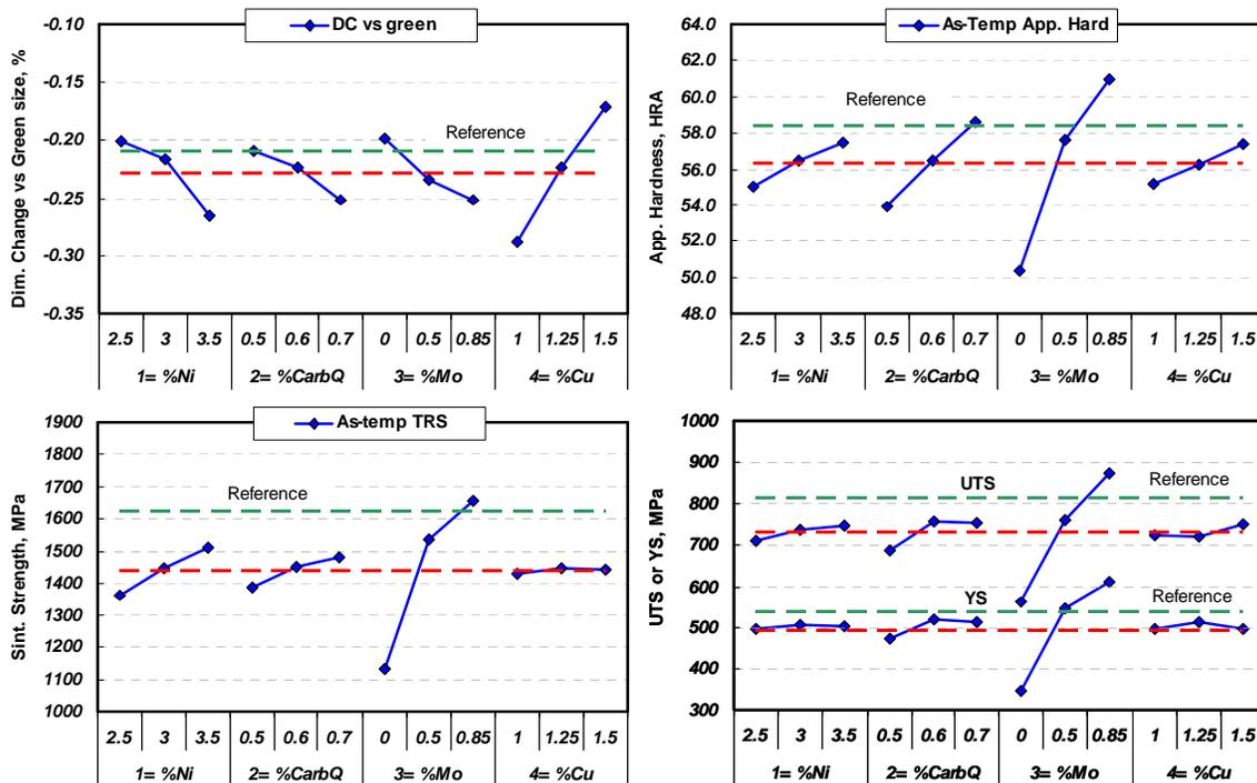
Figure 4. Effect of Ni, graphite (CarbQ), pre-alloyed Mo and Cu content on as-tempered properties at 7.0 g/cm<sup>3</sup>. Specimens were sintered at 1130°C and cooled under normal cooling rate (0.8°C/sec).
