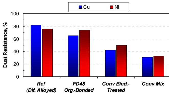
Figure 1. Ni and Cu dust resistance of various type of 4Ni-1.5Cu-0.5Mo steel powders.
