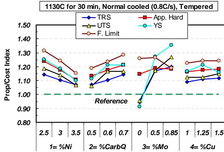
Figure 8. Effect of Ni, graphite, Mo and Cu content on the P/C Index (relative property to cost ratio) for standard sintering/cooling conditions after tempering.
