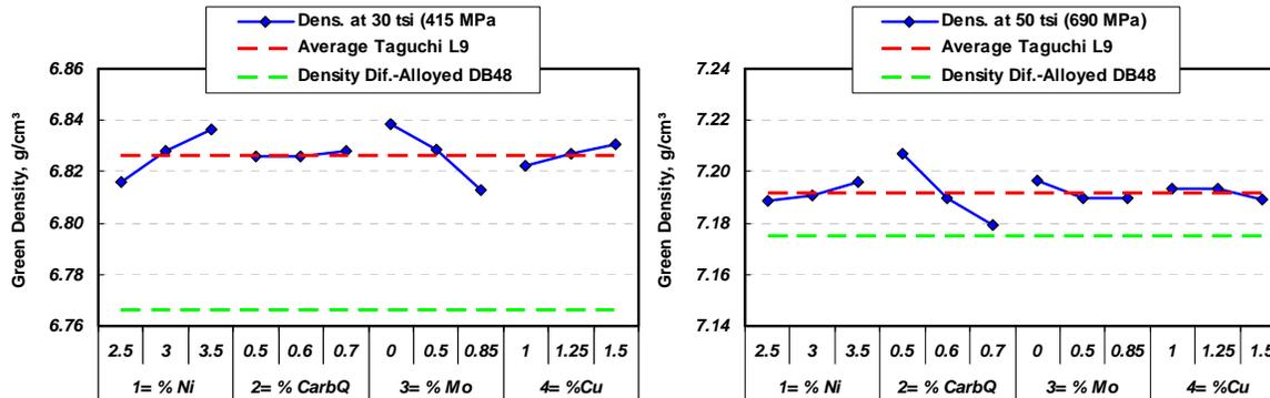
Figure 3. Effect of parameters on compressibility at 415 and 690 MPa (30 and 50 tsi).
