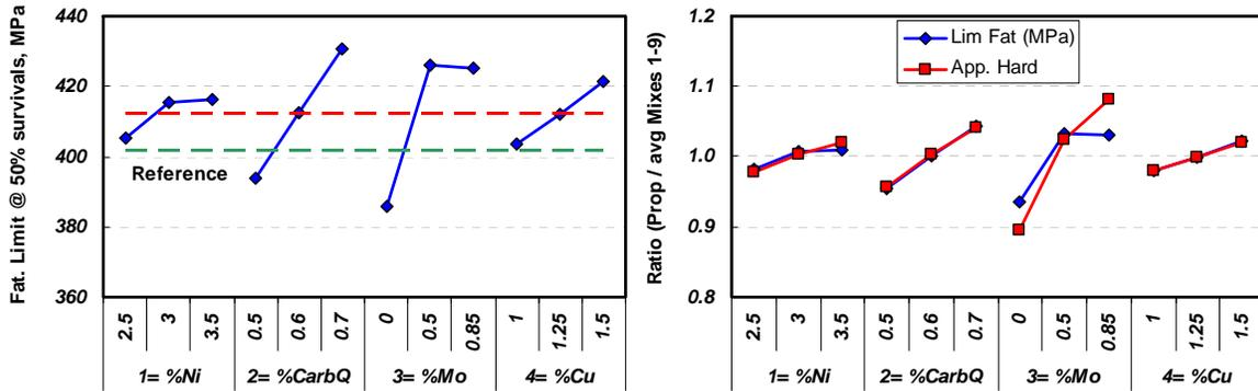
Figure 5. Effect of mix formulation on fatigue limit and apparent hardness.
