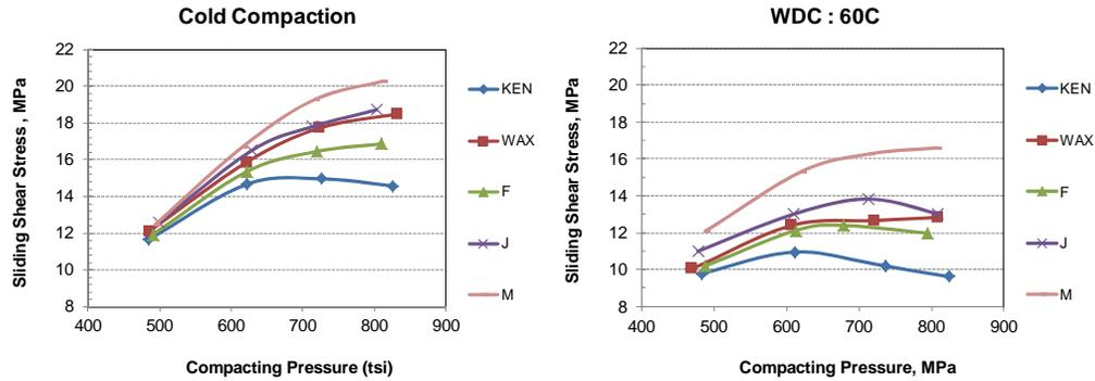
Fig. 7- Ejection performance (Sliding AVG) for Mixes F, J and M obtained by CC and WDC- 60°C (12.7 mm, 5 SPM).
