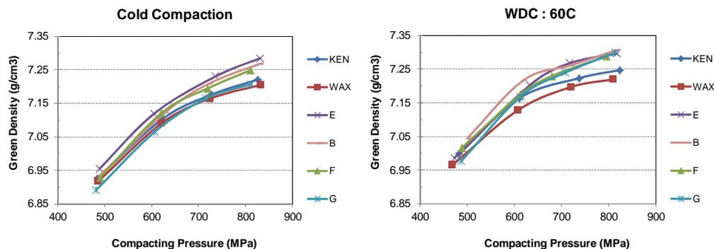
Fig. 1- Compressibility curves for group 2 obtained by CC and WDC- 60°C (12.7 mm, 5 SPM).
