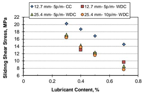
Fig. 10- Sliding shear stress versus the lubricant content.
