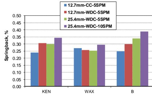
Fig. 11- Springback for different compacting conditions.
