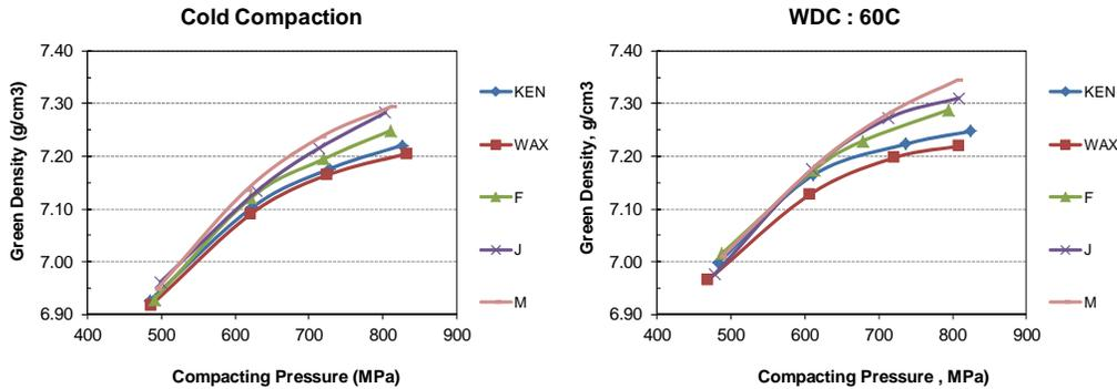
Fig. 6- Compressibility curves obtained for Mixes F, J and M obtained by CC and WDC- 60°C (12.7 mm, 5 SPM).
