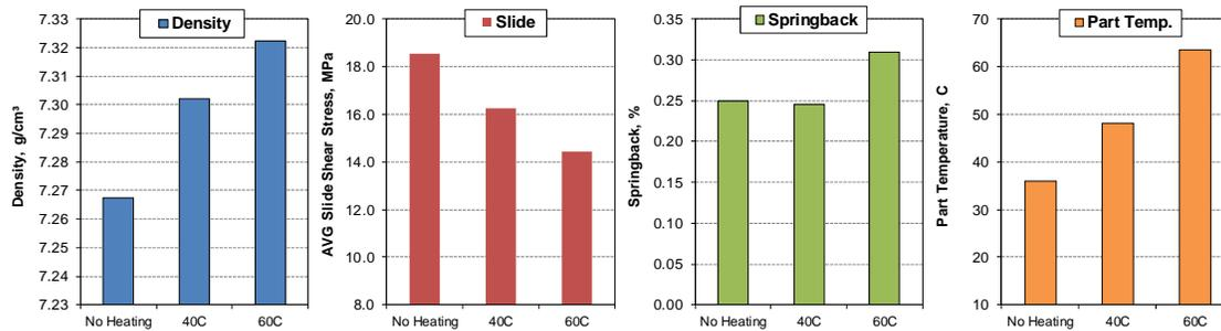
Fig. 12- Effect of die temperature on density, ejection slide shear stress and springback (12.7 mm, 5SPM)
