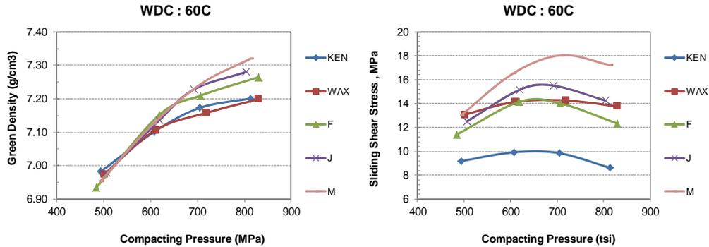
**Fig. 8- Green density and sliding shear stress as a function of compacting pressure for parts 25.4 mm tall (5 SPM).**
