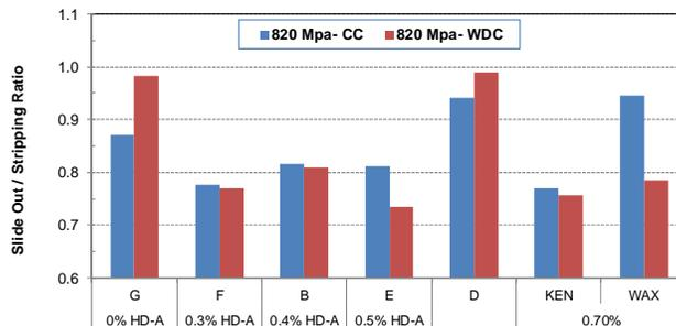
Fig. 5- Slide OUT/Stripping ratio for mixes pressed by CC and WDC at 60°C (12.7 mm, 5 SPM).
