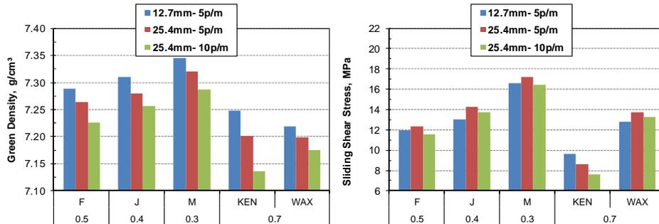
**Fig. 9- Comparison between tests carried out at 12.7 and 25.4 mm by WDC at 60°C and 820 MPa.**
