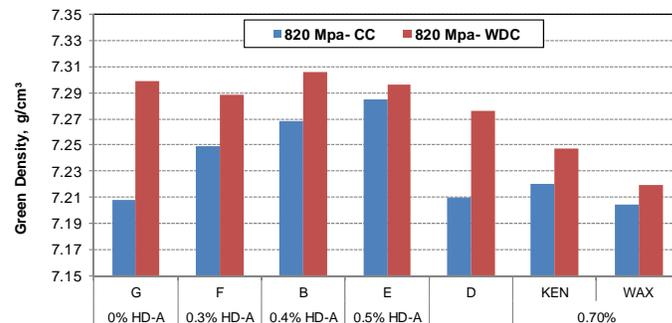
Fig. 2- Green density for different mixes at ~ 820 MPa (12.7 mm, 5 SPM).
