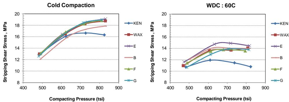
Fig. 3- Stripping shear stresses for specimens pressed by CC and WDC-60°C (12.7 mm, 5 SPM).
