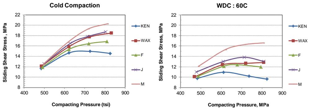
**Fig. 6- Ejection performance (Sliding AVG) for Mixes F, J and M obtained by CC and WDC- 60°C (12.7 mm, 5 SPM).**
