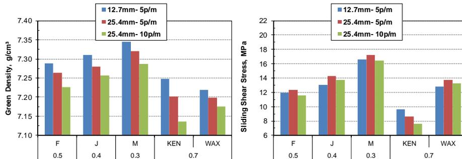
**Fig. 9- Comparison between tests carried out at 12.7 and 25.4 mm by WDC at 60°C and 820 MPa.**
