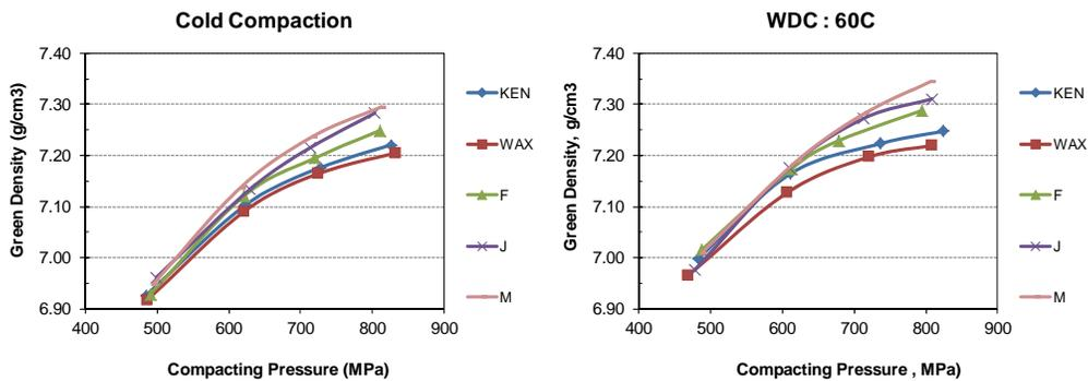
**Fig. 7- Compressibility curves obtained for Mixes F, J and M obtained by CC and WDC- 60°C (12.7 mm, 5 SPM).**
