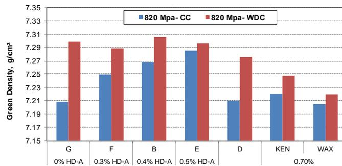
**Fig. 2- Green density for different mixes at ~ 820 MPa (12.7 mm, 5 SPM).**
