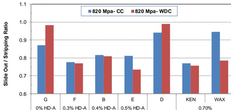
**Fig. 5- Slide OUT/Stripping ratio for mixes pressed by CC and DWC at 60°C (12.7 mm, 5 SPM).**
