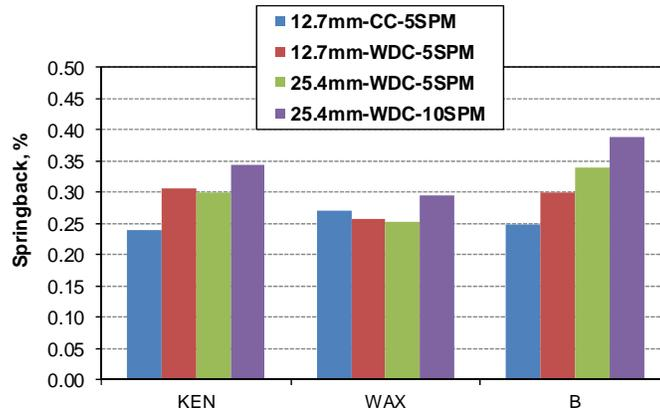
**Fig. 12- Springback for different compacting conditions (820 MPa).**
