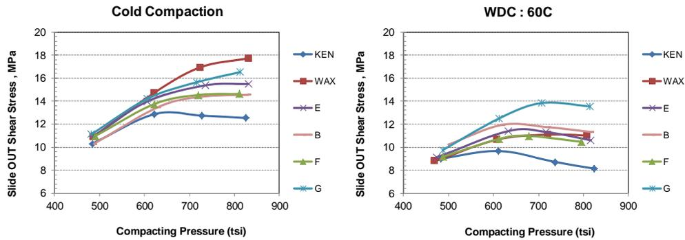
**Fig. 4- Slide OUT ejection shear stress for specimens pressed by CC and WDC-60°C (12.7 mm, 5 SPM).**
