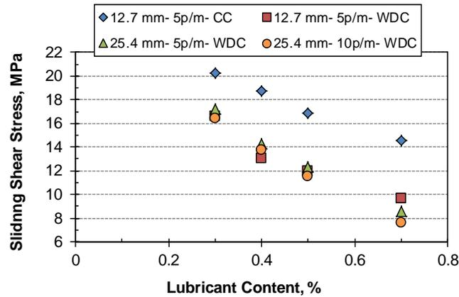
**Fig. 10- Sliding shear stress versus the lubricant content.**
