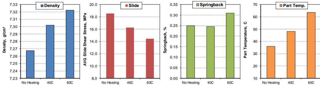
**Fig. 11- Effect of die temperature on density, ejection slide shear stress and springback (12.7 mm, 5SPM)**
