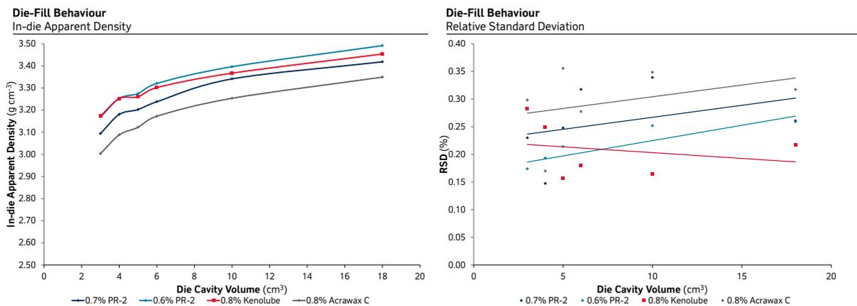
**Figure 1.** Die-fill behaviour of the various mixes.
