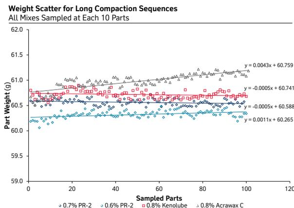
**Figure 2.** Evolution of the part weight measured throughout the long compaction sequences.
