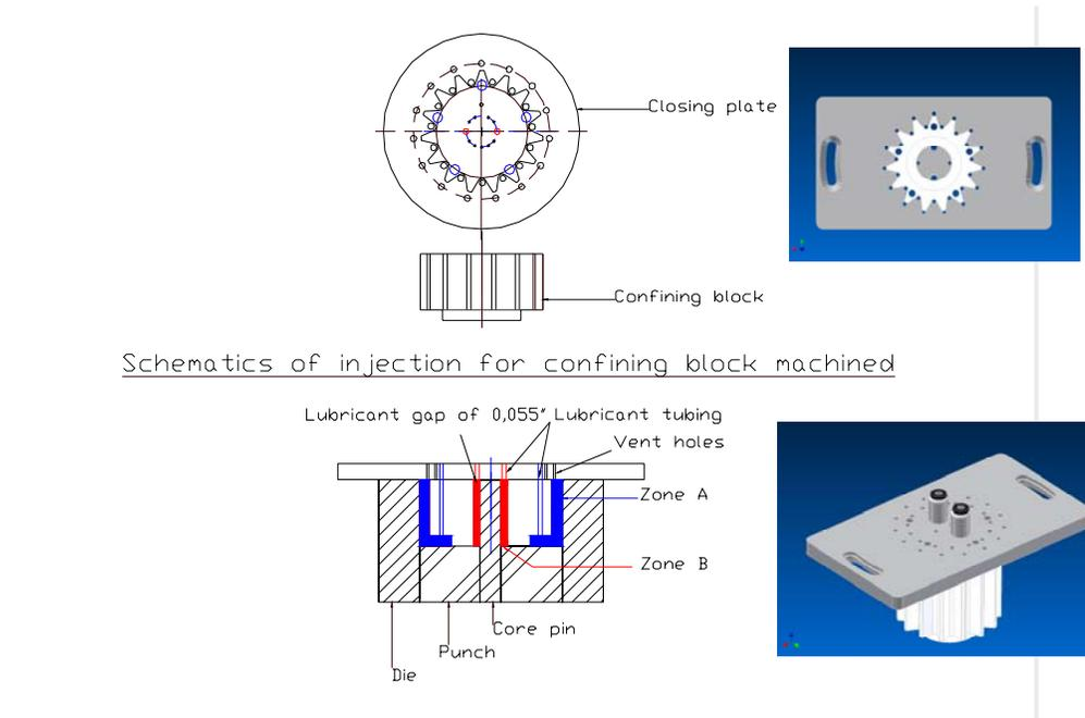
**Figure 4:** Drawing of the spraying unit (confining block and closing plate) used to apply lubricant both on die walls and core pin when processing gears #1.
