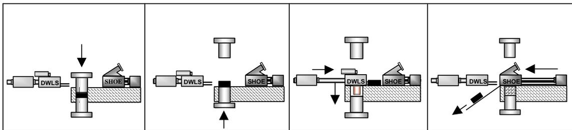
**Figure 13:** DWL system configuration where the spraying unit actuator is independent of the feed shoe.
