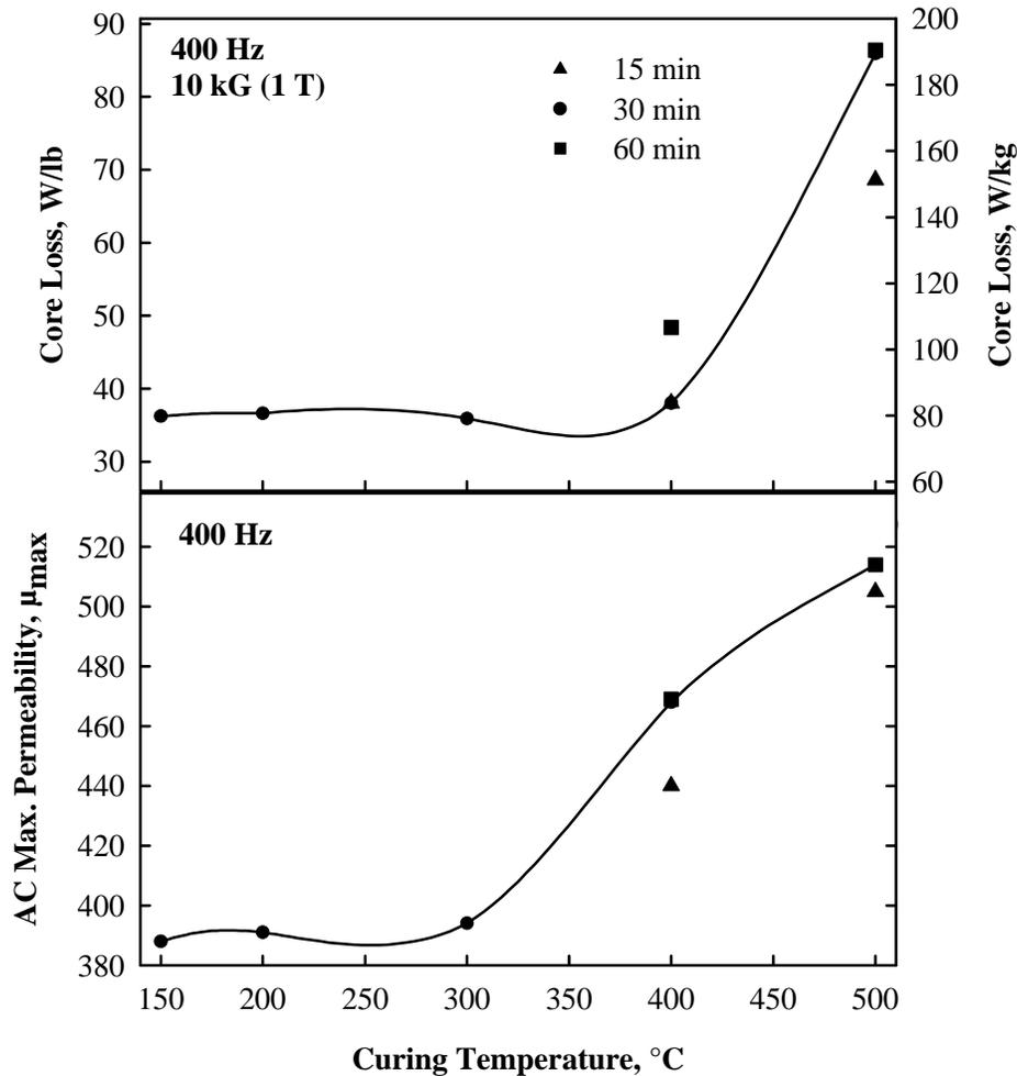
Figure 8. Effect of curing time and temperature on core loss at 10 kG (1 T) and AC maximum permeability at 400 Hz.
