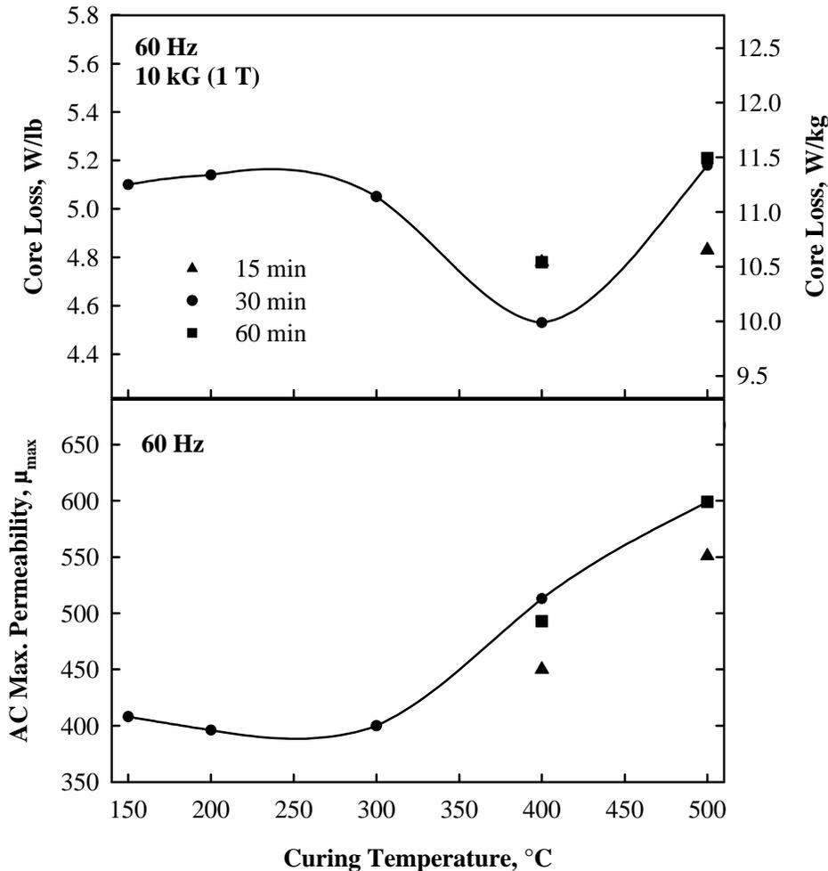
Figure 7. Effect of curing time and temperature on core loss at 10 kG (1 T) and AC maximum permeability at 60 Hz.
