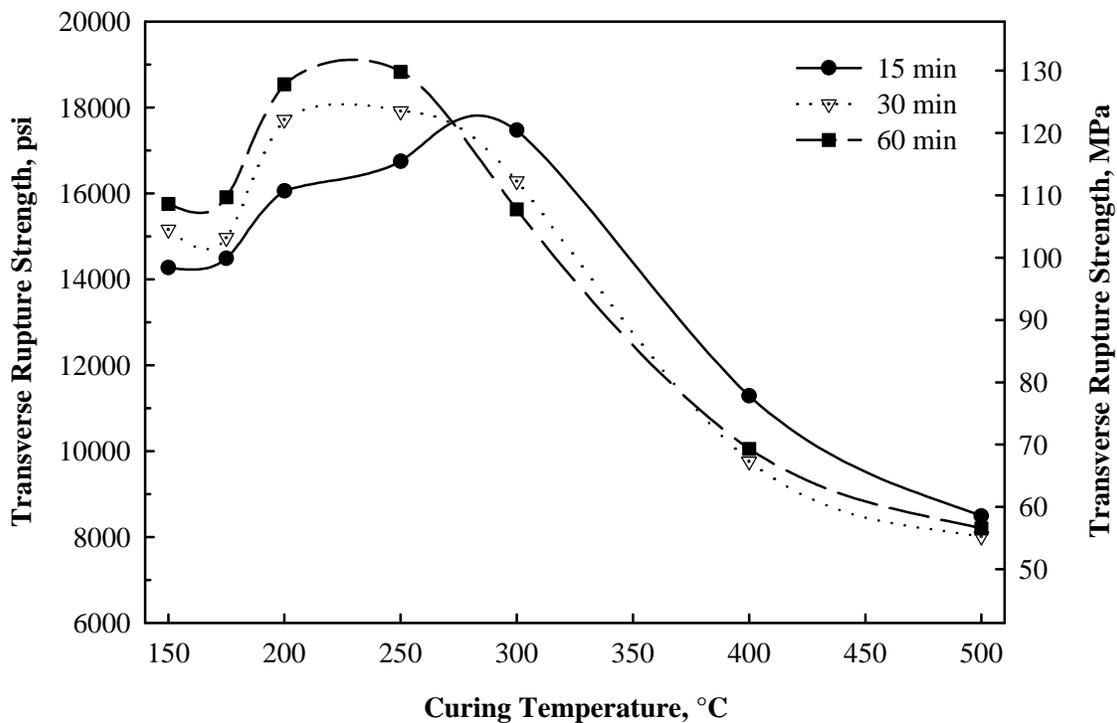
Figure 1. Effect of curing temperature and time on the mechanical strength of iron/0.8% resin composites pressed at 620 MPa (45 tsi) and 65°C.
