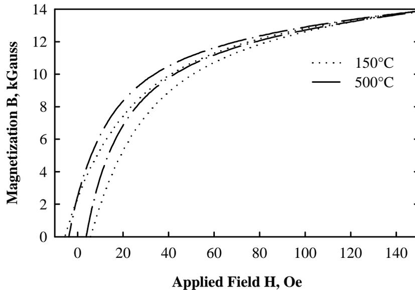
Figure 4. First half of the magnetization loop at an applied field of 150 Oe (11940 A/m) for iron/0.8% resin rings cured for 30 minutes at 150°C and 500°C.
