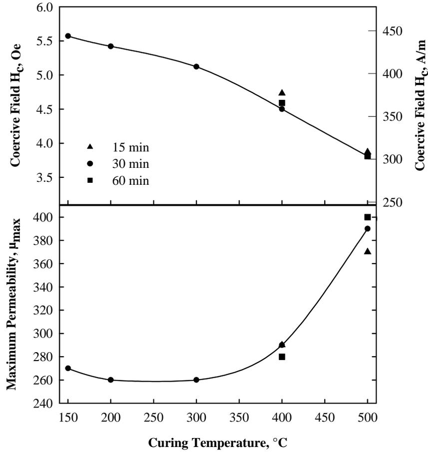
Figure 5. Effect of curing temperature and time on  $H_c$  and  $\mu_{max}$  measured in a 150 Oe applied field (11940 A/m) for iron/0.8% resin composites pressed at 620 MPa (45 tsi) and 65°C.
