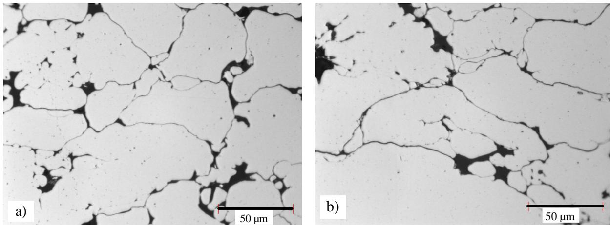
Figure 3. Optical micrographs of iron/0.8% resin composites pressed at 620 MPa (45 tsi) and 65°C and cured in air for 30 minutes at two temperatures: a) 175°C and b) 500°C.
