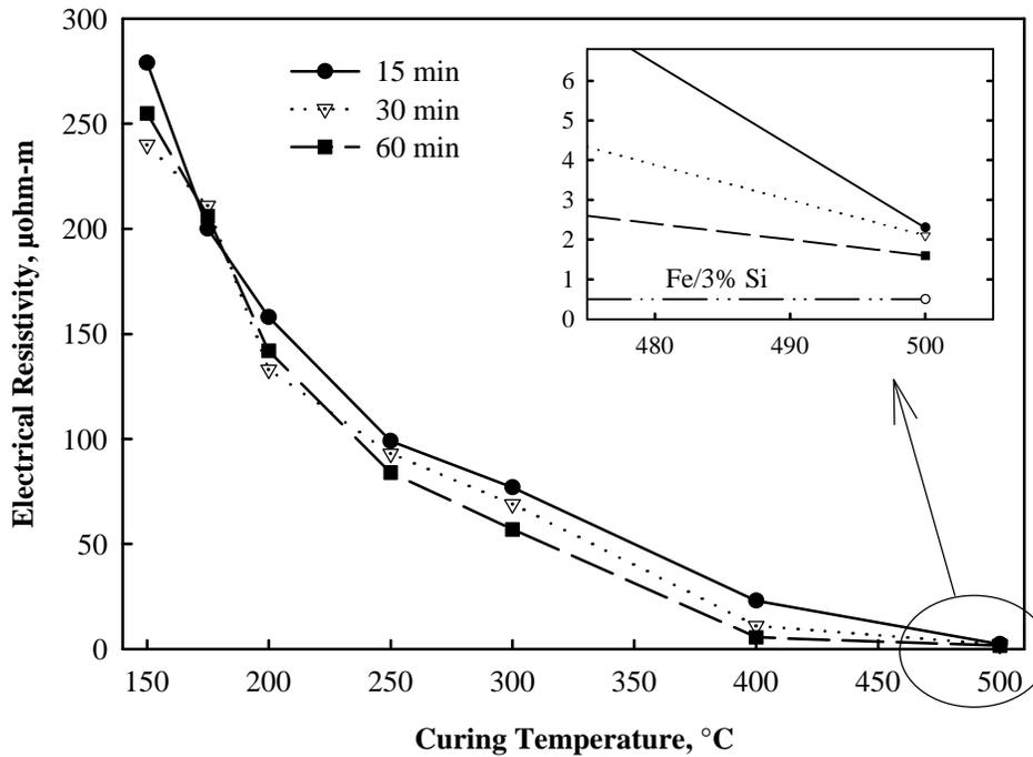
Figure 2. Effect of curing temperature and time on the electrical resistivity of iron/0.8% resin composites pressed at 620 MPa (45 tsi) and 65°C.
