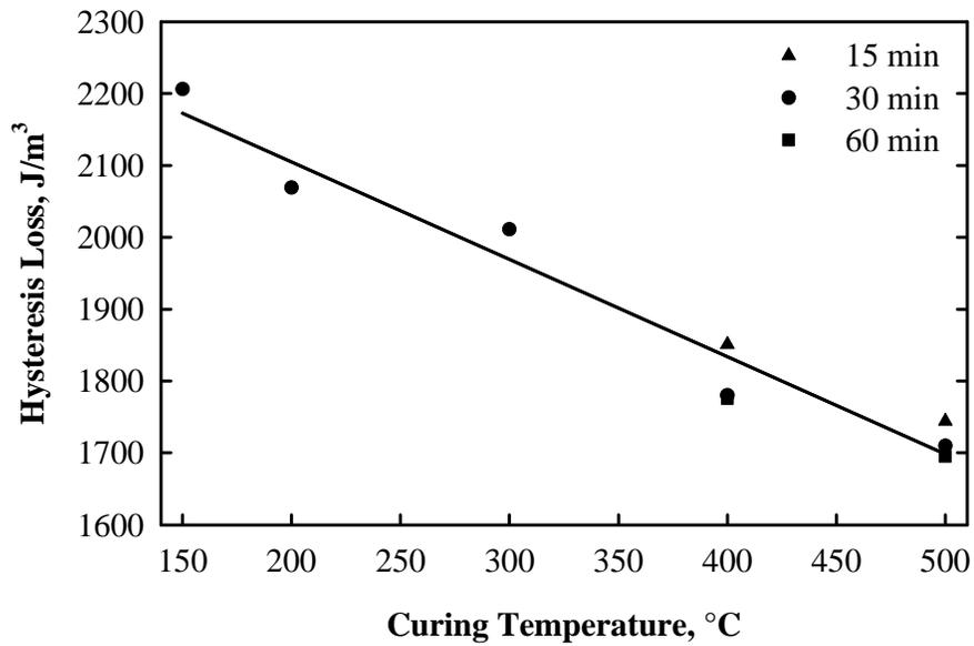
Figure 6. Effect of the curing time and temperature on the hysteresis loss of iron/0.8% resin composites pressed at 620 MPa (45 tsi) and 65°C.
