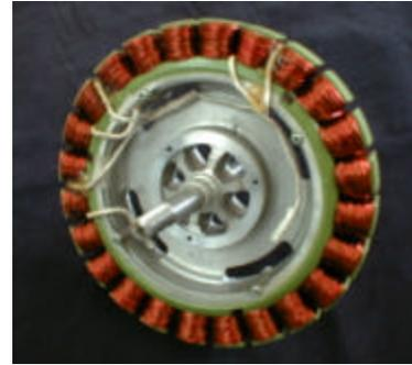
**Figure 13.** Final SMC stator comprising four segments inserted between two aluminum flanges.
