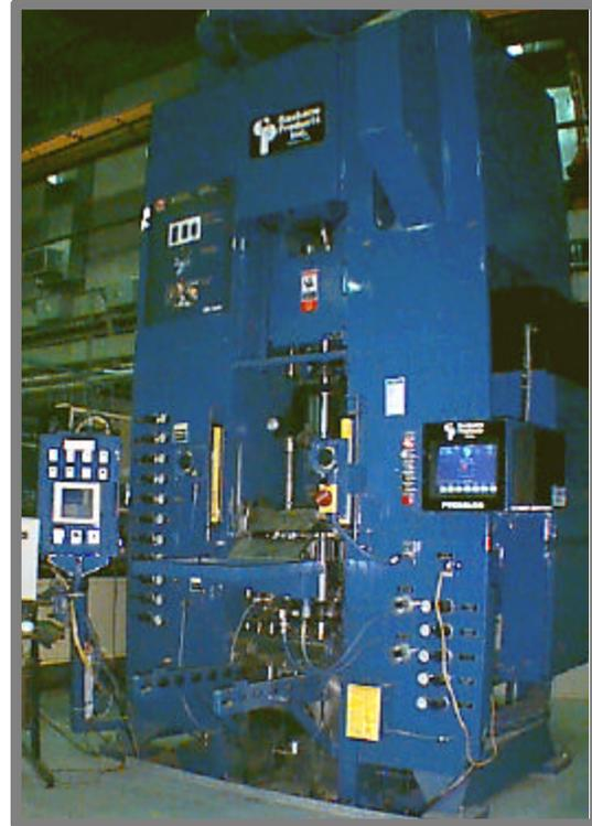
**Figure 9 :** Mechanical press used in the prototyping.
