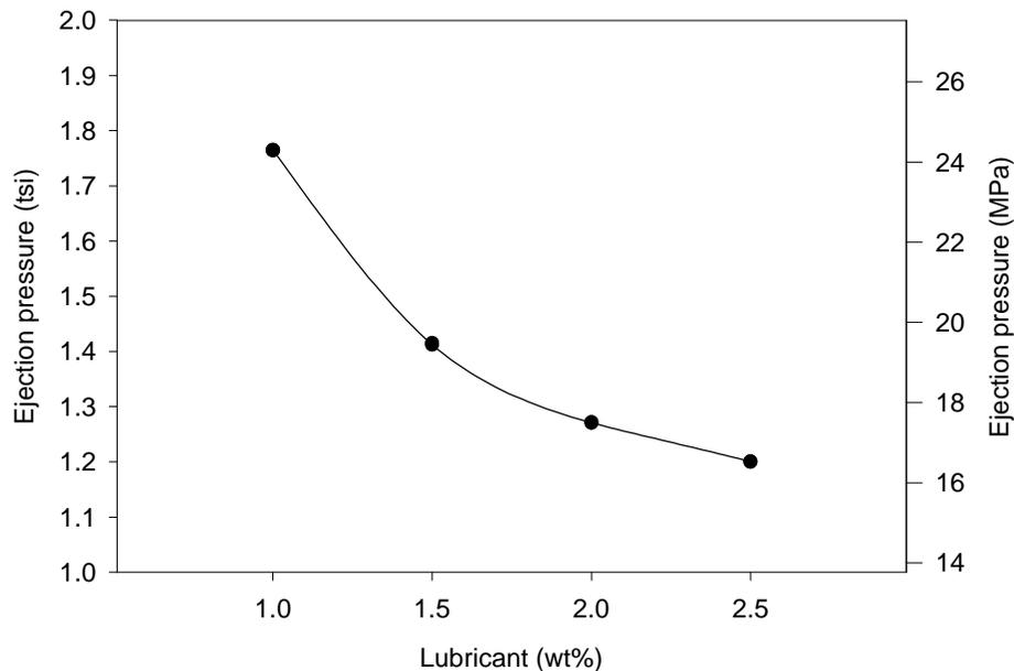
**Figure 1.** Effect of lubricant content on peak ejection pressure of TRS bars pressed at 620 MPa (45 tsi).
