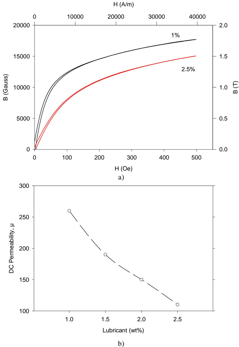
**Figure 4.** Effect of lubricant content on DC magnetic properties: a) DC magnetization curves and b) DC maximum permeability.
