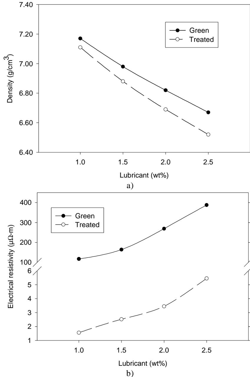
**Figure 2.** Effect of lubricant content on a) density and b) electrical resistivity of TRS bars before and after a thermal treatment at 600°C.
