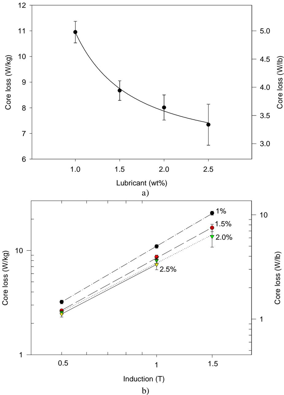
**Figure 5.** Effect of lubricant content on core loss at 60 Hz: a) for an induction of 1 T and b) at different inductions.
