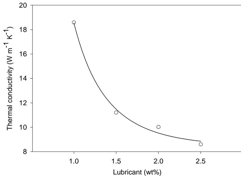
**Figure 3.** Effect of the lubricant content on the thermal conductivity of thermal-treated bars after resin impregnation.
