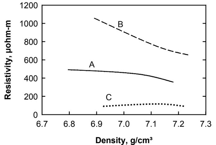
Figure 4. Effect of density on the bulk resistivity of the three materials as determined on TR bars cured 30 min in air : material A at 200°C, B at 160°C and C at 350°C.
