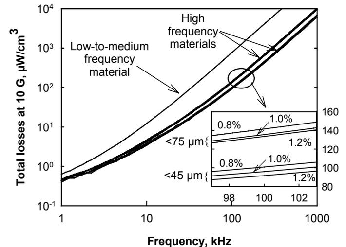
Figure 8. Total losses at 1 mT for high frequency materials compared with a low-to-medium frequency material. The inset at 100 kHz shows the effect of the iron particle size and resin content.
