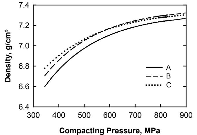
Figure 1. Effect of compacting pressure on the density of TR bars pressed from the three composite materials.
