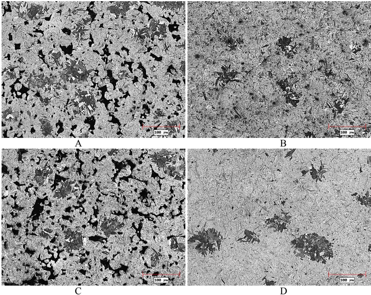
Figure 2. Microstructure of specimens after etching (Nital 2%).
