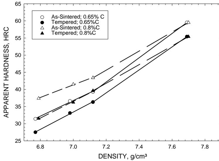
Figure 1. Effect of density and carbon content on apparent hardness of sinter hardened specimens in the as-sintered condition and after tempering 60 minutes in air at 205°C.
