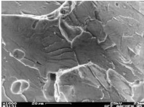
Fig. 9. Shear fracture surface of surface of MSP 3.5 Mo at +150°C
