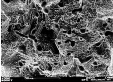
Fig. 12. Reproduction of a fracture in the middle of a case hardened sample (T = RT)
