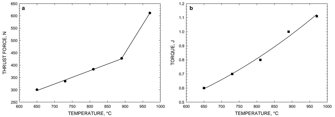
**Figure 3. Effect of Pre-Sintering Temperature on Average Thrust Force (a) and Torque (b).**
