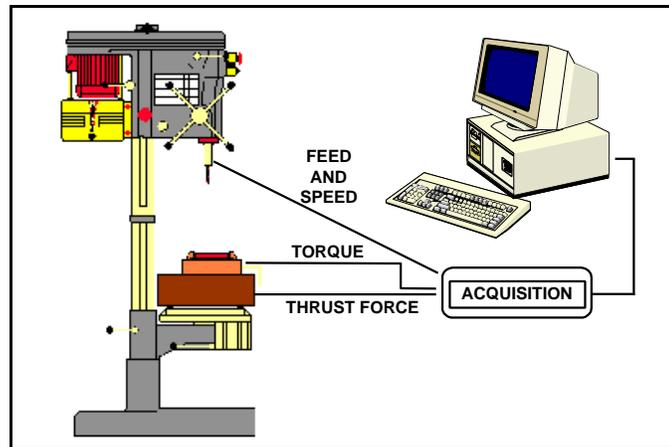
**Figure 1. Set-up Used to Evaluate Drilling Thrust Force and Torque.**
