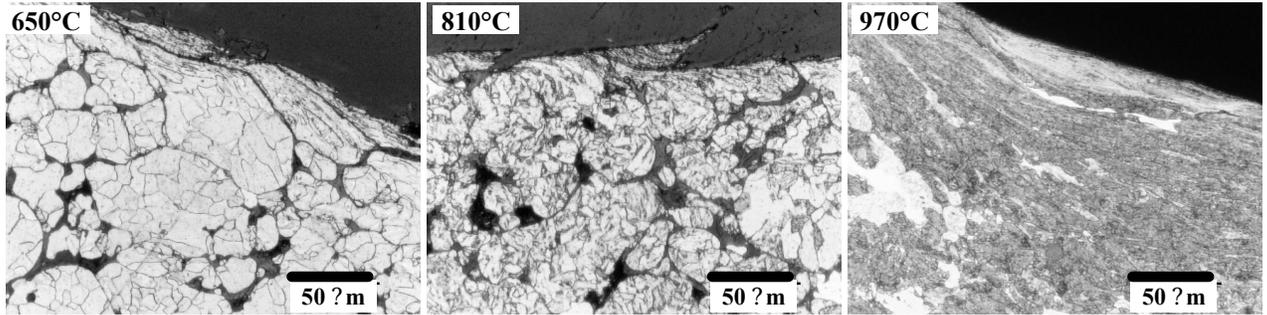
**Figure 6. Surface Under the Cut of Specimens Made from ATOMET 4701 with 0.9% Graphite, 2% Cu at 6.8 g/cm<sup>3</sup> for Pre-Sintering Temperatures of 650, 810 and 970°C.**
