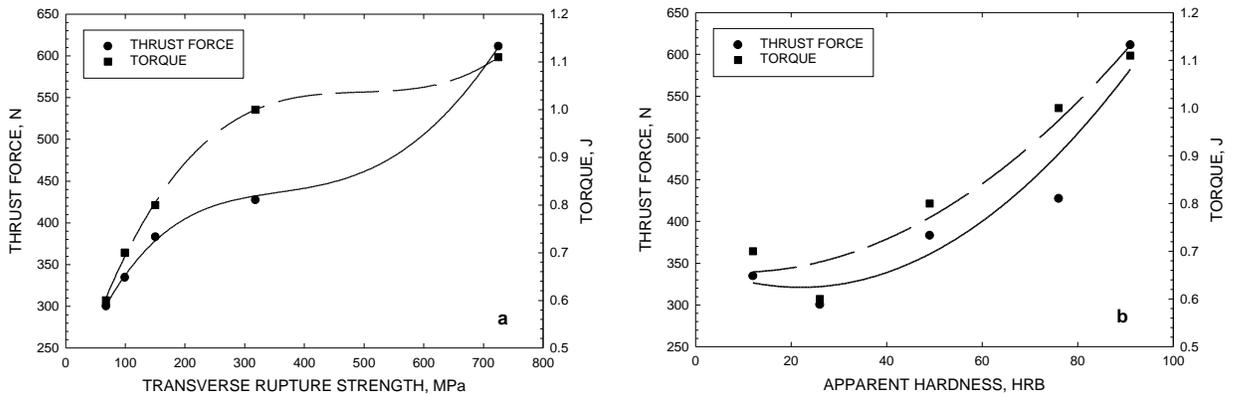
**Figure 4. Relationship Between Transverse Rupture Strength (a) and Apparent Hardness (b) with the Average Thrust Force and Torque Required to Drill 15 Holes.**
