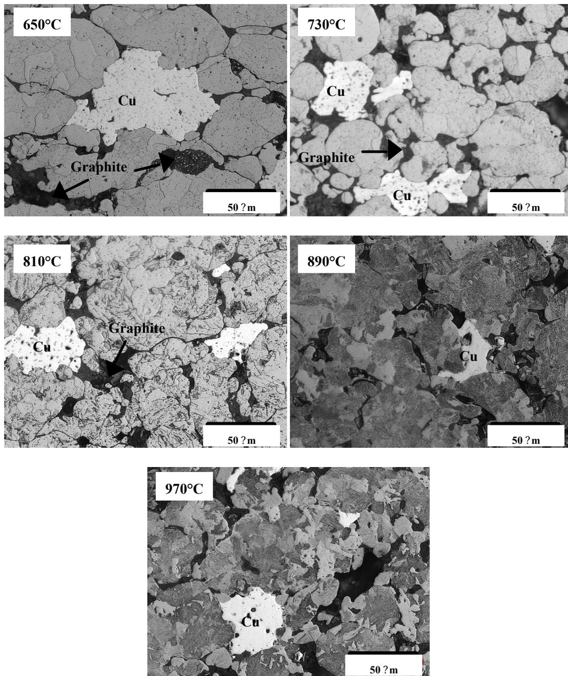
**Figure 5. Microstructures of Specimens Made from ATOMET 4701 with 0.9% Graphite, 2% Cu at 6.8 g/cm<sup>3</sup> After Pre-Sintering Treatments.**
