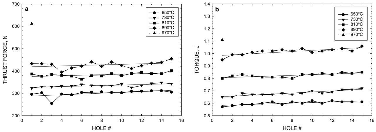
**Figure 2. Average Thrust Force (a) and Torque (b) Measurements When drilling Holes in Specimens Pre-Sintered at 650, 730, 810, 890 and 970°C.**
