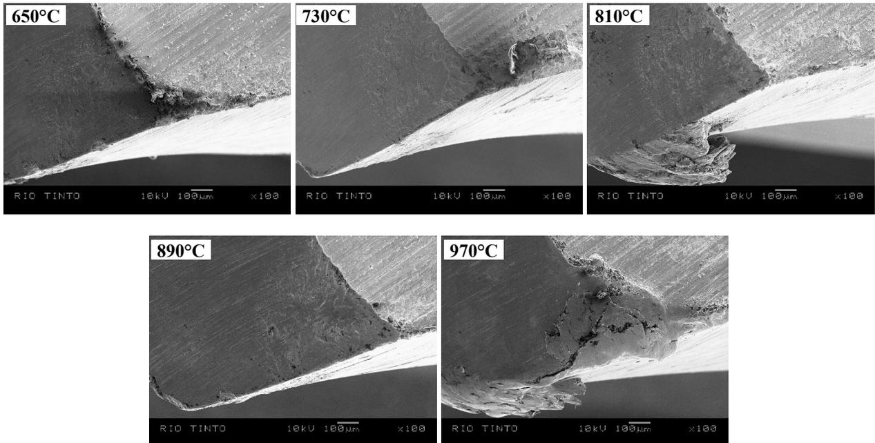
**Figure 7. Tool Wear Developed on the Drills for the Specimens Made from ATOMET 4701 with 0.9% Graphite, 2% Cu at 6.8 g/cm<sup>3</sup> at Various Pre-Sintering Temperatures.**
