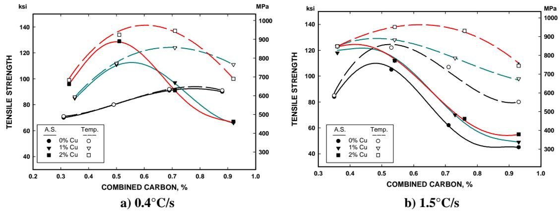
Figure 8. Evolution of Tensile Strength as a Function of the Combined Carbon and Copper Concentrations for Cooling rates of a) 0.4°C/s and b) 1.5°C/s in the Temperature Range of 650 to 400°C (Specimens Pressed to a Green Density of 6.9 g/cm<sup>3</sup>).
