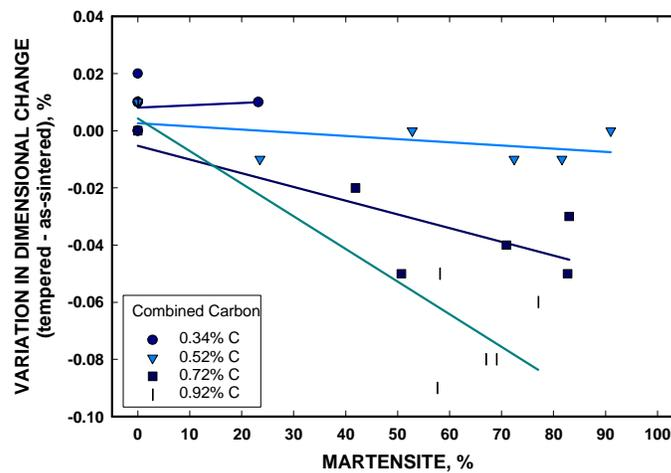
Figure 7. Difference in Dimensional Change Between the As-Sintered and Tempered Conditions of Sinter Hardened Specimens as a Function of the Martensite and Combined Carbon Concentration (Specimens Pressed to a Green Density of 6.9 g/cm<sup>3</sup>).
