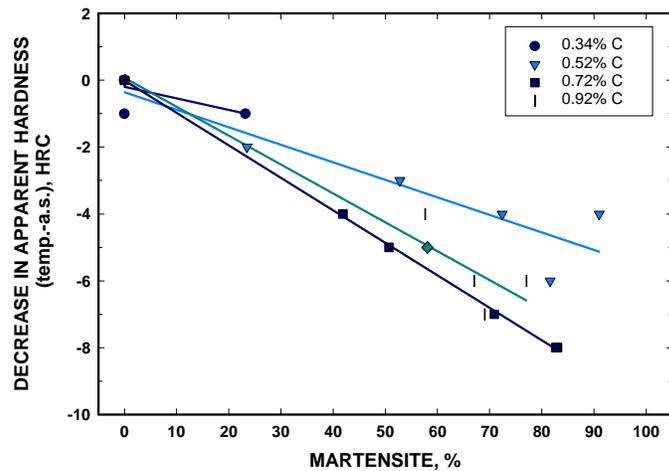
Figure 5. Loss in Apparent Hardness After Tempering at 200°C as a Function of Martensite and Combined Carbon in Sinter Hardened P/M Steels (Specimens Pressed to a Green Density of 6.9 g/cm<sup>3</sup>).
