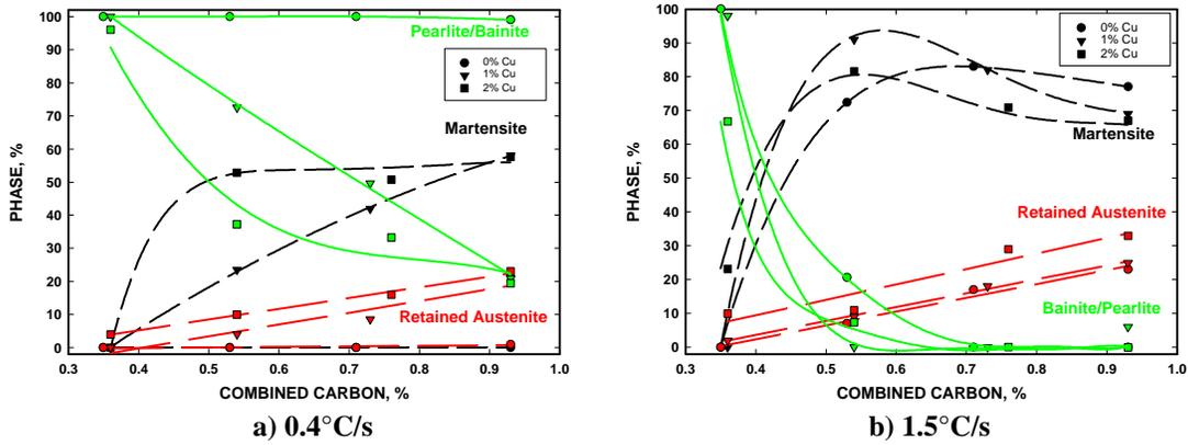
Figure 3. Variation of the Relative Amount of Martensite, Retained Austenite and Pearlite/Bainite as a Function of Combined Carbon and Copper Concentrations for Cooling Rates of a) 0.4°C/s and b) 1.5°C/s in the Temperature Range of 650 to 400°C (Specimens Pressed to a Green Density of 6.9 g/cm<sup>3</sup>).
