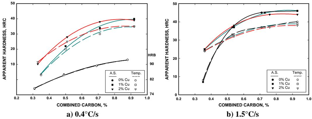
Figure 1. Effect of Combined Carbon and Copper Concentrations on Apparent Hardness of Specimens Cooled at a) 0.4°C/s and b) 1.5°C/s in the Temperature Range of 650 to 400°C (Specimens Pressed to a Green Density of 6.9 g/cm<sup>3</sup>).
