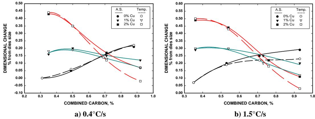
Figure 6. Evolution of Dimensional Change from Die Size as a Function of the Combined Carbon and Copper Concentrations for Cooling Rates of a) 0.4°C/s and b) 1.5°C/s in the Temperature Range of 650 to 400°C (Specimens Pressed to a Green Density of 6.9 g/cm<sup>3</sup>).
