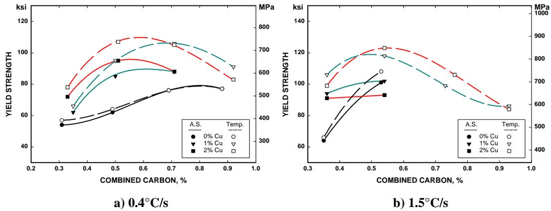
Figure 9. Evolution of Yield Strength as a Function of the Combined Carbon and Copper Concentrations for Cooling Rates of 0.4 and 1.5°C/s in the Temperature Range of 650 to 400°C (Specimens Pressed to a Green Density of 6.9 g/cm<sup>3</sup>).
