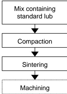
Figure 1. Typical Flow Diagram of a Conventional P/M Process Using Standard Lubricants.
