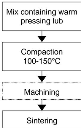
Figure 7. Typical Flow Diagram of the Warm Compaction Process.
