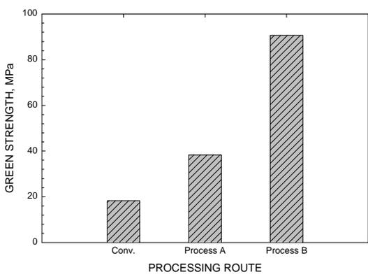
Figure 11. Green Strength of Specimens Pressed to 7.10 g/cm<sup>3</sup> (F-0005 Mixes Containing 0.75% Lubricant).
