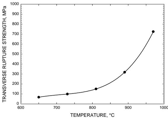
Figure 4. Effect of Pre-Sintering Temperature on the Strength of Specimens Pressed to 6.8 g/cm<sup>3</sup> (ATOMET 4701+0.9% graphite+2% copper).
