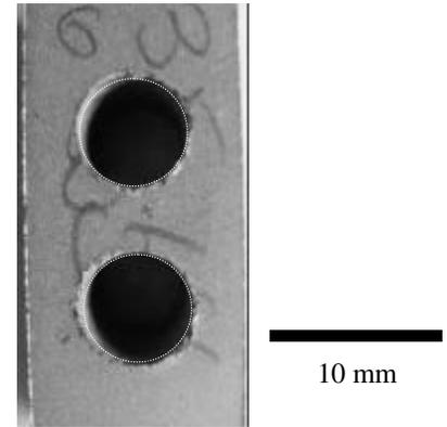
Made with ATOMET 4701+0.90% Graphite+2% Copper+0.75% Wax Pressed to 6.8 g/cm<sup>3</sup> and Pre-Sintered 28 Minutes at 810°C.
