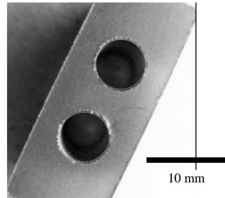
Figure 9. Breakout as the Drill Exited a Specimen Made from a FN-0205 Mix Pressed at 690 MPa and 130°C (Green Density; 7.35 g/cm<sup>3</sup>).
