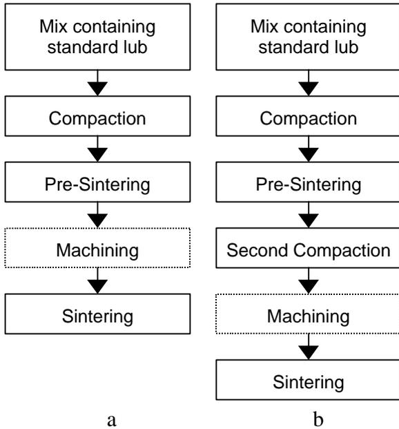
Figure 3. Flow Diagrams of Processes where Machining Can Be Carried Out after a Pre-Sintering Operation.
