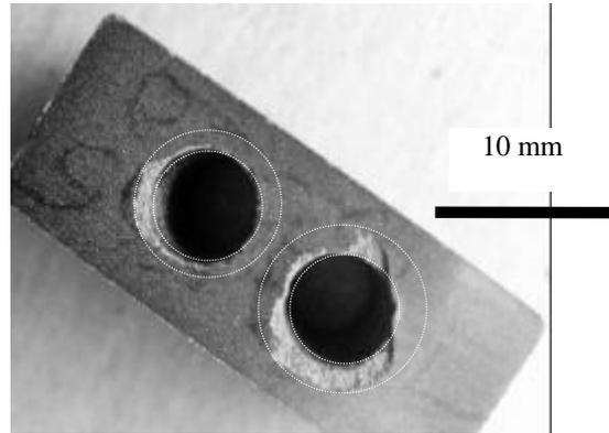
Figure 2. Breakout as the Drill Exited a Specimen Made from a F-0005 Mix Containing 0.75% Wax and Pressed to a Density of 7.10 g/cm<sup>3</sup>.
