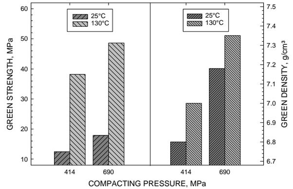
Figure 8. Effect of Compacting Pressure and Temperature on Green strength and Green Density (Specimens Pressed from FN-0205 mixes containing 0.6% Lubricant).
