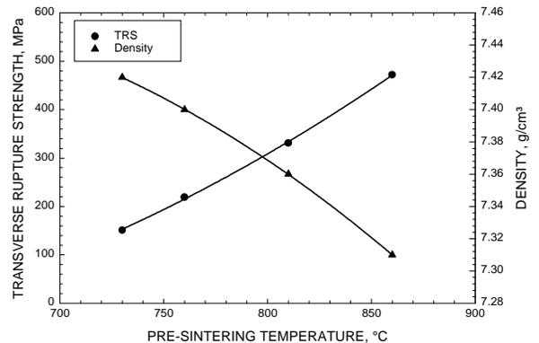
Figure 6. Strength and Density of FLN4-4405 Specimens After Pressing at 690 MPa and Re-Pressing at 690 MPa Vs Pre-Sintering Temperature.
