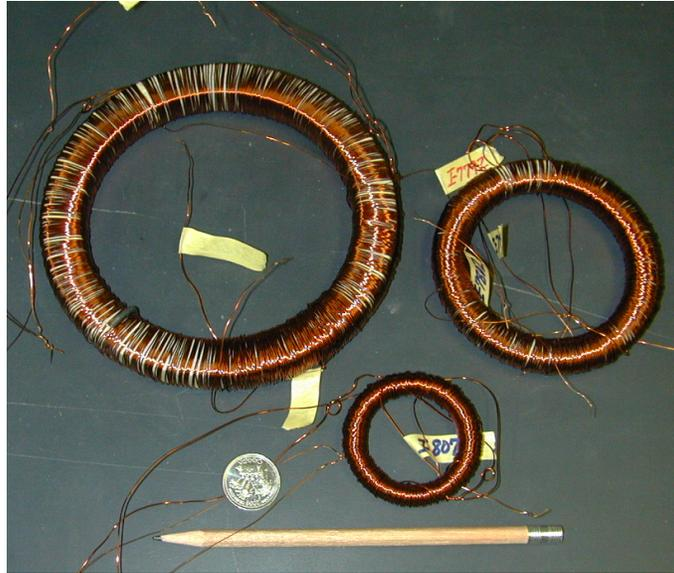
**Figure 1:** Three different rings wound for magnetic characterization.
