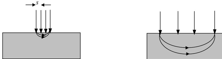
**Figure 9:** Effect of probe spacing on the penetration of the electric current and the volume analyzed.
