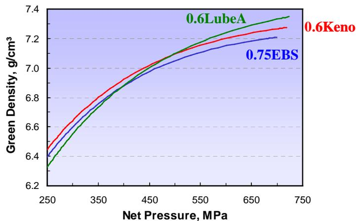
**Figure 7.** True compressibility curves for FN0205 mixes containing 0.6% Kenolube, 0.6% Lube A and 0.75% EBS wax pressed at 60°C.
