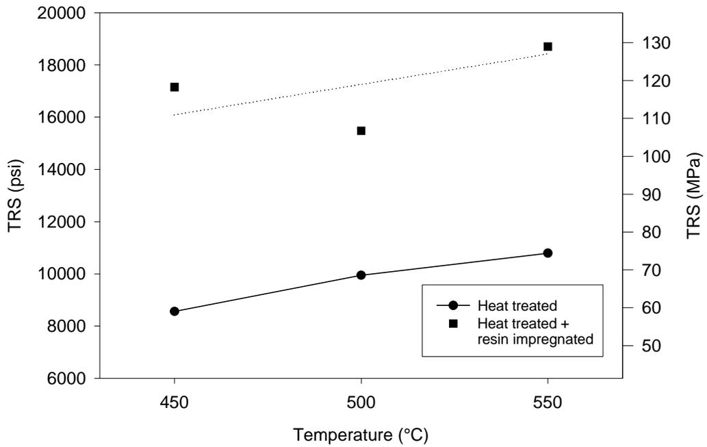
**Figure 8.** Effect of the thermal treatment temperature (30 min in N<sub>2</sub>) on the strength before and after resin-impregnation of bars compacted at 620 MPa/65°C.
