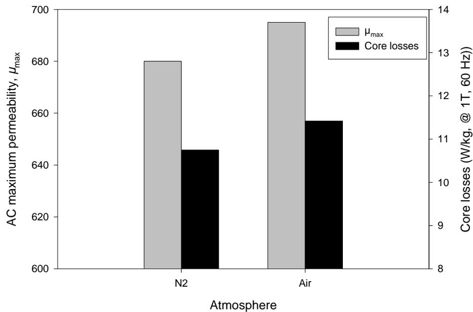
**Figure 5.** Effect of the thermal treatment atmosphere on the AC maximum permeability at 60 Hz and core losses (at 60 Hz/1 T) for rings pressed at 620 MPa/65°C, heated 30 min at 500°C and resin-impregnated.
