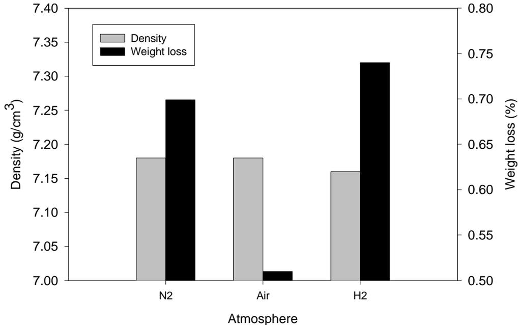
**Figure 1.** Effect of the thermal treatment atmosphere (30 min at 500°C) on the density and weight loss of iron/0.75% EBS bars compacted at 620 MPa/65°C.
