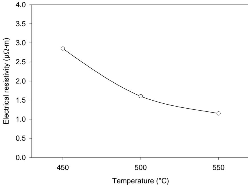
**Figure 7.** Effect of the thermal treatment temperature (30 min in N<sub>2</sub>) on the electrical resistivity of bars compacted at 620 MPa/65°C.
