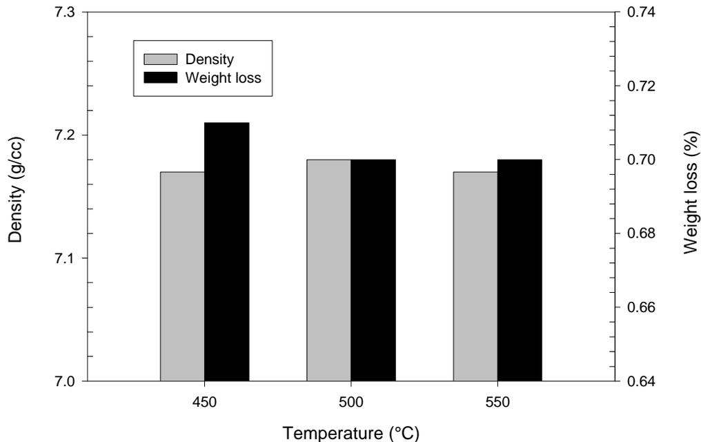
**Figure 6.** Effect of the thermal treatment temperature (30 min in N<sub>2</sub>) on the density and weight loss of TRS bars compacted at 620 MPa/65°C.
