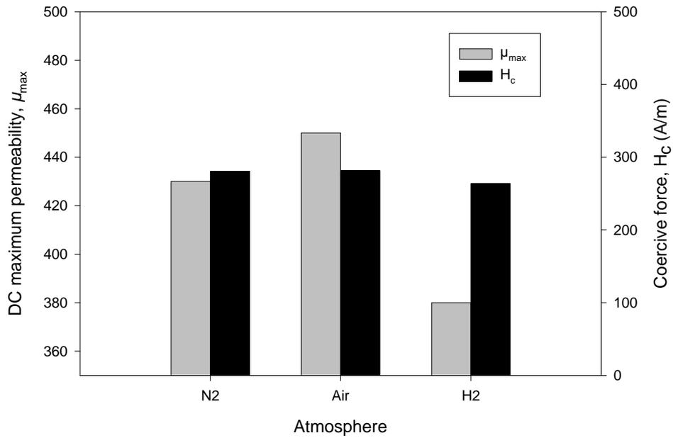
**Figure 4.** Effect of the thermal treatment atmosphere on the DC maximum permeability and coercive force ( $B = 11.9$  kA/m or 150 Oe) for rings pressed at 620 MPa/65°C, heated at 500°C for 30 min and resin-impregnated.
