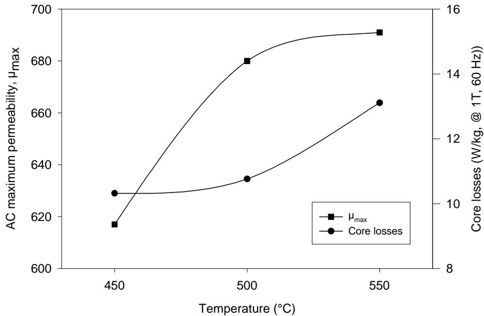
**Figure 10.** Effect of the thermal treatment temperature (30 min in N<sub>2</sub>) on the AC maximum permeability at 60 Hz and core losses (1 T/60 Hz) of rings compacted at 65°C/620 MPa.
