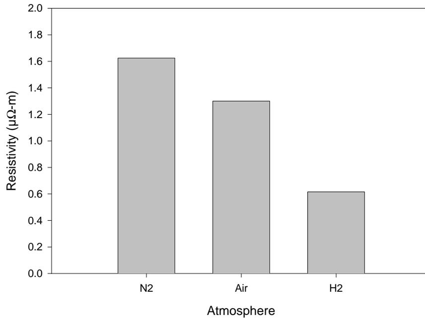
**Figure 2.** Effect of the thermal treatment atmosphere (30 min at 500°C) on the electrical resistivity of iron/0.75% EBS bars compacted at 620 MPa/65°C.
