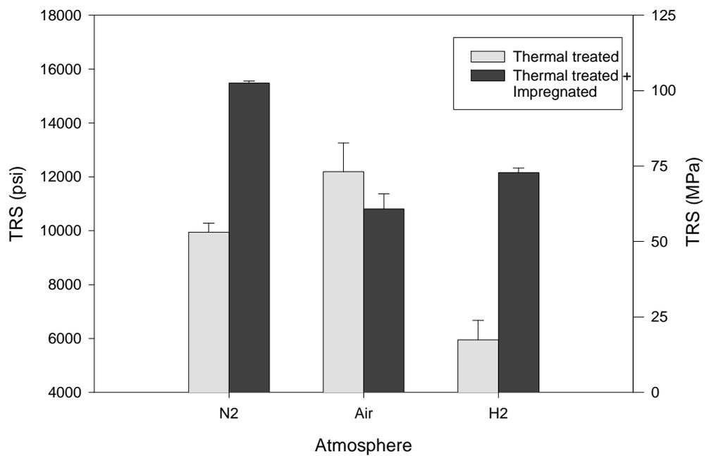
**Figure 3.** Effect of the thermal treatment atmosphere (30 min at 500°C) on the strength before and after resin-impregnation (iron/0.75% EBS bars compacted at 620 MPa/65°C).
