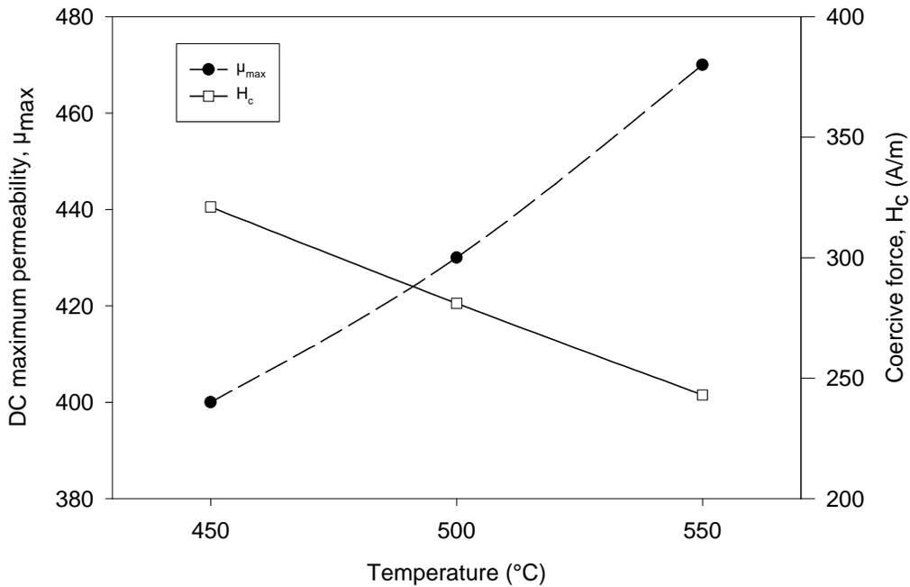
**Figure 9.** Effect of the thermal treatment temperature (30 min in N<sub>2</sub>) on maximum permeability and coercive force  $H_c$  ( $B = 11.9$  kA/m or 150 Oe) of rings compacted at 620 MPa/65°C.
