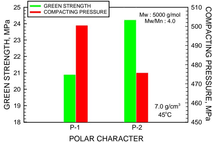
Figure 4. Effect of the Polar Character of the Functional Groups of a Polymeric Type Lubricant on Green Properties. (P-1 < P-2)
