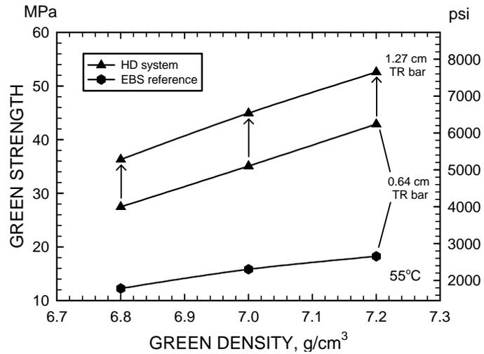
Figure 8. Green Strength of Specimens Pressed from the HD System and the EBS Reference as a Function of Green Density.
