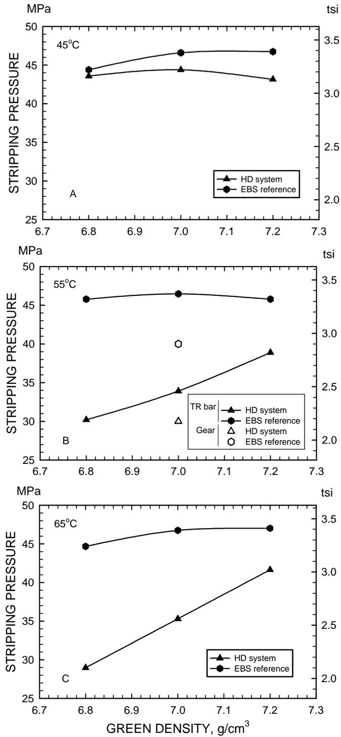
Figure 6. Stripping Pressure Required to Eject Specimens Containing the New HD Lubricating System or Conventional EBS Reference on Lab (TR bar) and Production (Gear) Presses at Various Temperatures.
