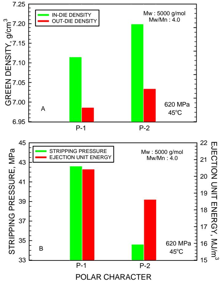
Figure 3. Effect of the Polar Character of the Functional Groups of a Polymeric Type Lubricant on Green Density, Stripping Pressure and Ejection Unit Energy. (P-1 < P-2)
