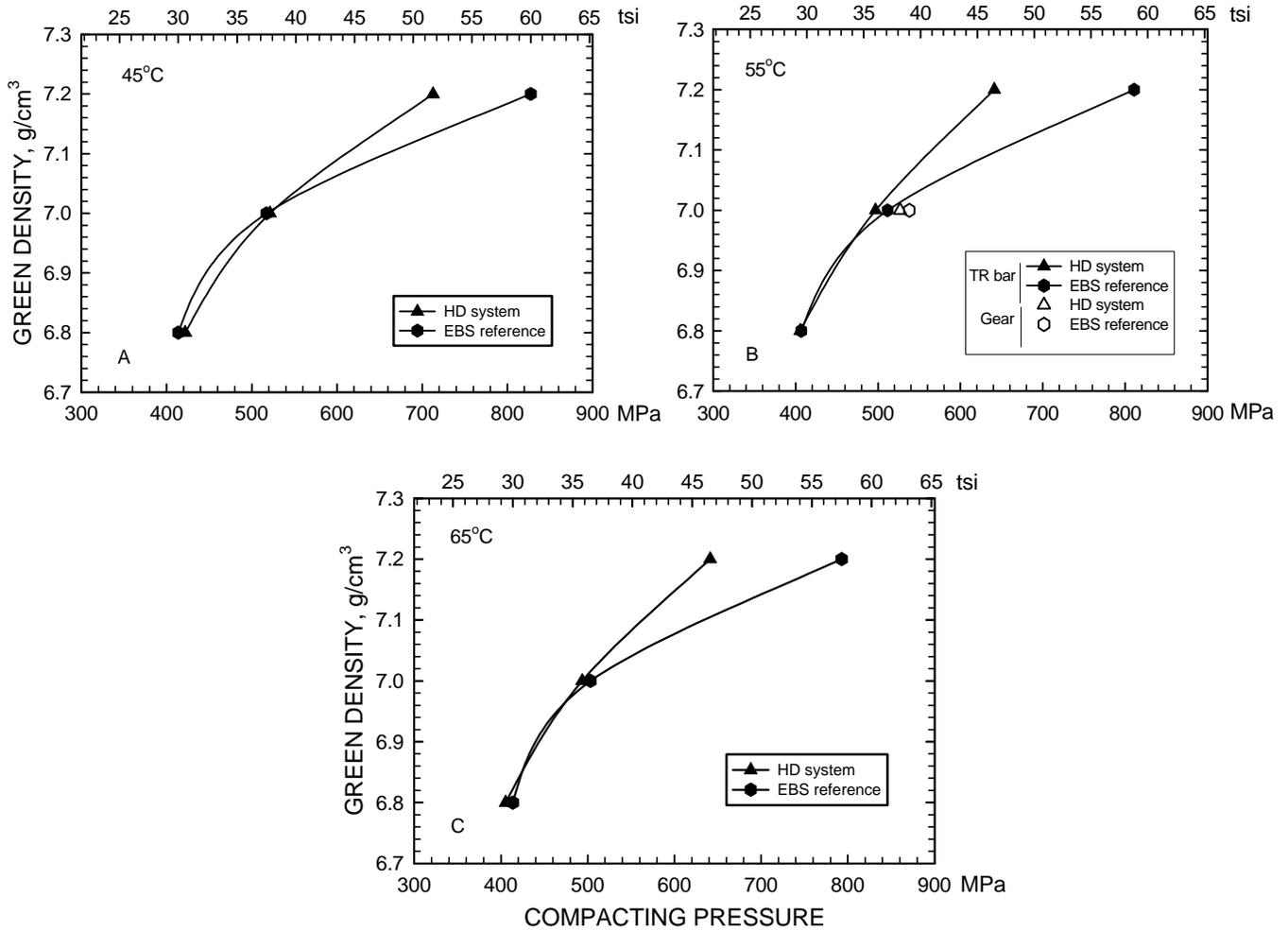
Figure 5. Compressibility of Mixes Containing HD and EBS Lubricating Systems on Lab and Production Presses at Various Compacting Temperatures.
