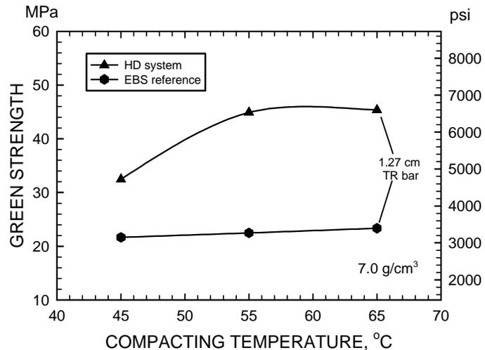
Figure 9. Green Strength of Specimens Pressed from the HD System and the EBS Reference as a Function of the Compacting Temperature.
