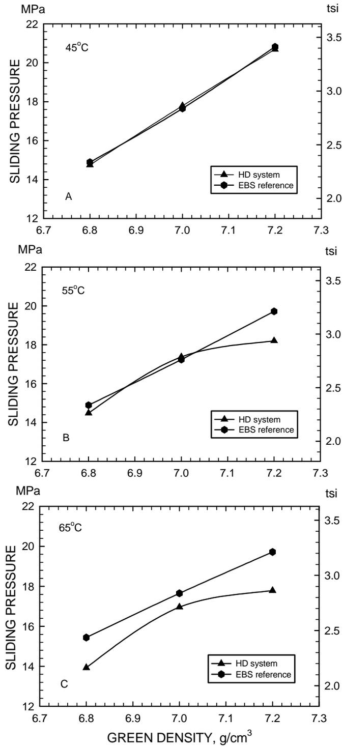
Figure 7. Sliding Pressure Required to Eject Specimens Containing the New HD Lubricating System or Conventional EBS Reference on a Lab Press at Various Temperatures.
