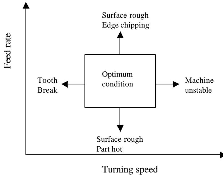
Figure 5. Processing window for green machining operation.
