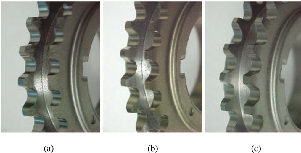
Figure 3. Surface finish of green machined parts at turning speed of 750 rpm and feed rate of 0.07 mm/rev. (a) As-Compacted, (b) Cured and (c) Pre-Sintered
