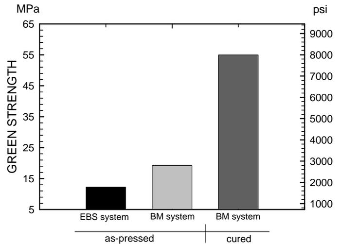
Figure 6. Effect of the curing treatment on green strength of 0.64 cm thick specimens pressed from the BM system and comparison with the EBS system.
