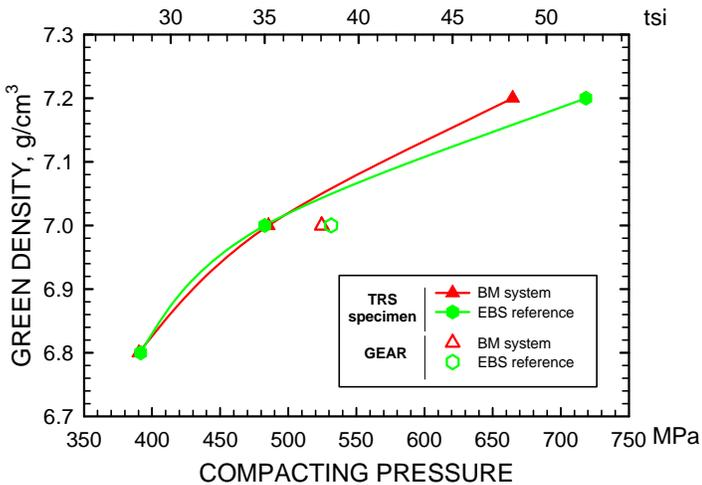
Figure 3. Compressibility of mixes containing BM and EBS lubricating systems on lab and production presses.
