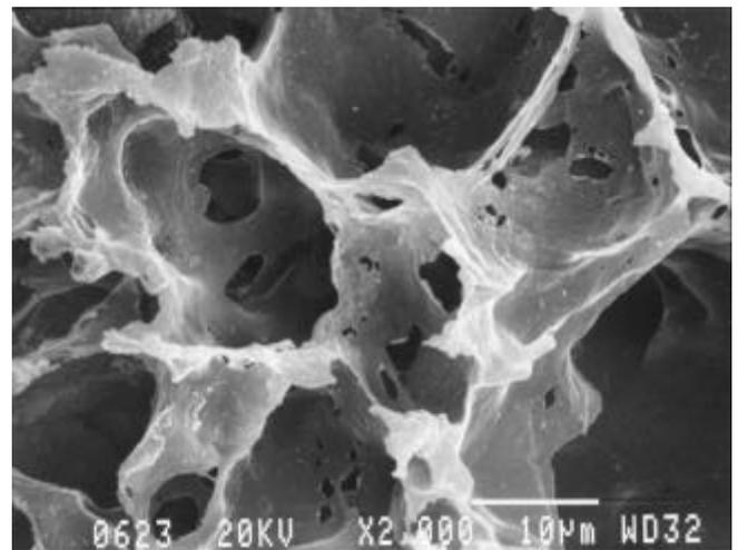
Figure 7. Illustration of the thin network of lubricant throughout cured TRS specimens pressed from the BM system.
