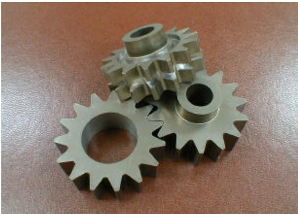
Figure 13. Examples of industrial machining on gears cured at 175°C for 1 hour.
