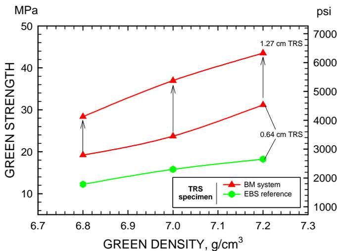
Figure 5. Green strength of specimens pressed from the BM system and the EBS reference as a function of green density.
