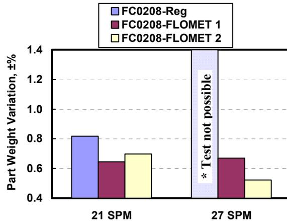
**Figure 13.** Part weight variation obtained during production runs with regular and binder-treated mixes. \* The regular FC0208 mix was not run at 27 SPM because of a too large variation.
