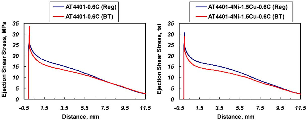
**Figure 15.** Ejection curves for FL-4405 and FLN4-4405-1.5% Cu mixes. EBS Wax content : 0.65%. AT1001 and AT4440 refer to ATOMET 1001 and ATOMET 4401 respectively.
