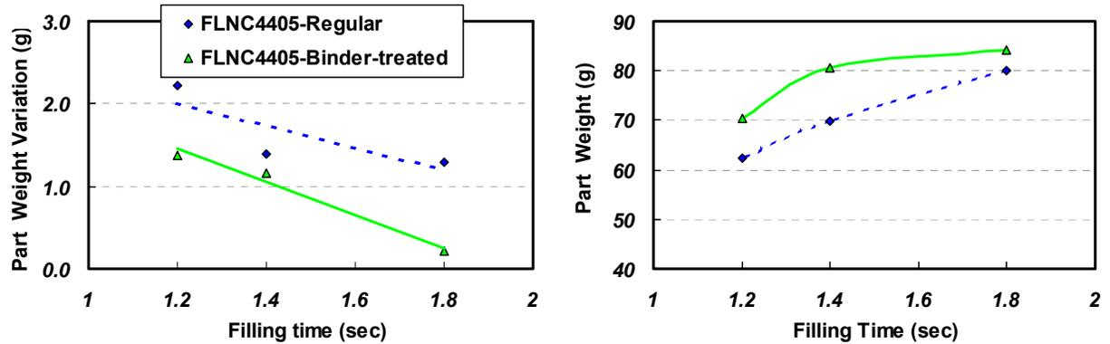
**Figure 12.** Results of test #2 carried out in the *gravity fill mode* under more difficult filling conditions (fill height/wall thickness = 8.2).
