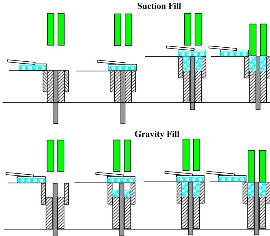
**Figure 9.** Illustration of the two modes of die cavity filling used in a mechanical press.
