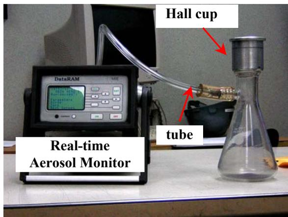
**Figure 6.** Experimental assembly used to evaluate the dust created during the flow of powder mixes.
