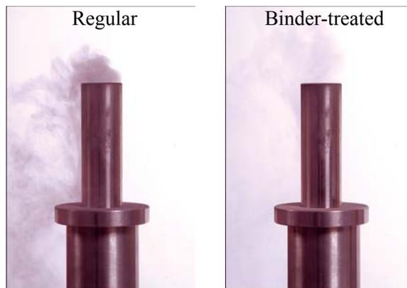
**Figure 5.** Dust produced with regular and binder-treated mixes in an apparatus used to measure resistance to dusting (6 liter/min air flow through a 25 mm diameter tube).
