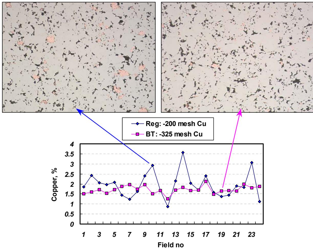
**Figure 16.** Distribution of copper in specimens made of FC0208 mixes. Regular mix (Reg) contains a -200 mesh Cu while the binder-treated mix (BT) contains a -325 mesh Cu grade.
