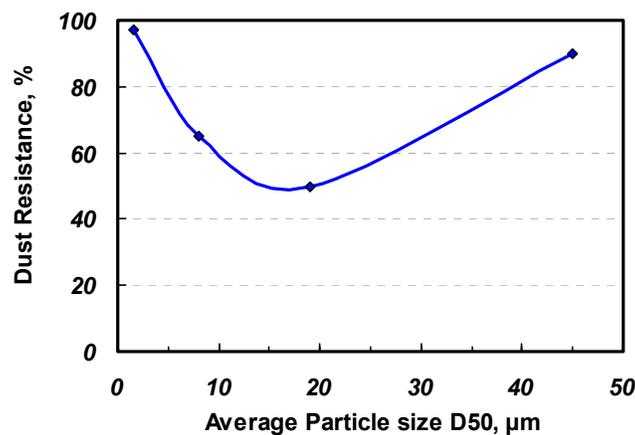
**Figure 8.** Effect of mean particle size D<sub>50</sub> of metallic additives on the dust resistance after binder-treatment.
