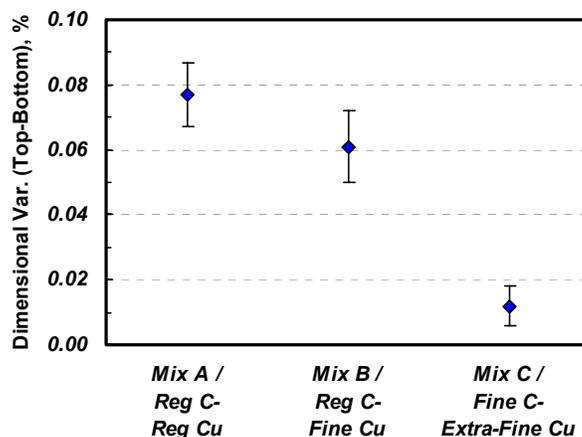
**Figure 17.** Dimensional variation between the top and the bottom of rings made of FLN4-4405 mixes containing different grades of Cu and graphite. Mixes contain 2.6% Cu.
