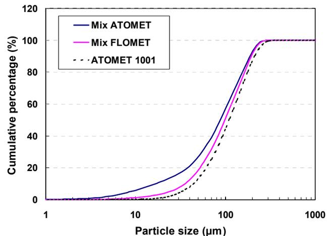
**Figure 4.** Particle size distribution of regular and binder-treated FLOMET mixes (laser particle analyzer). ATOMET 1001 + 2%Ni + 0.85% C + 0.75% EBS wax
