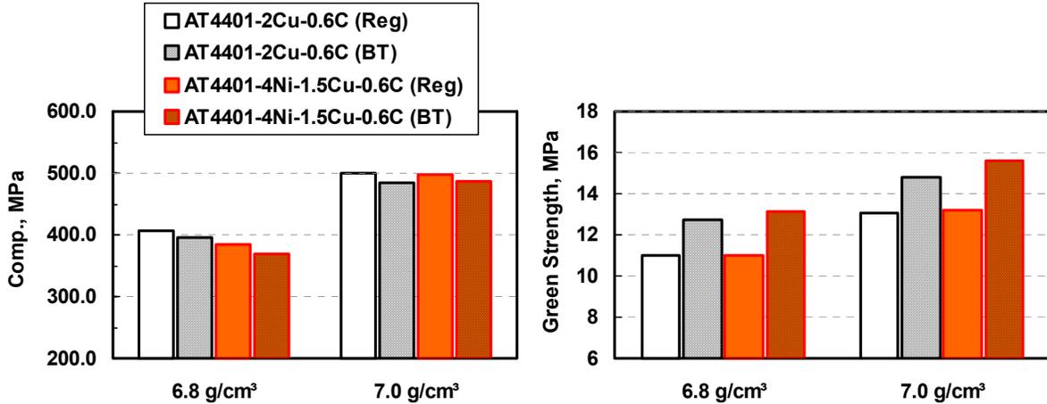
**Figure 14.** Compacting pressure and green strength achieved at 6.8 and 7.0 g/cm<sup>3</sup> with two different mix formulations. Specimens pressed at 60°C. AT1001 and AT4440 refer to ATOMET 1001 and ATOMET 4401 respectively.
