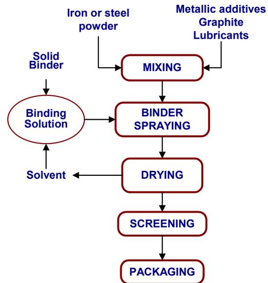
**Figure 1.** Process flow diagram of the binder-treatment technology.
