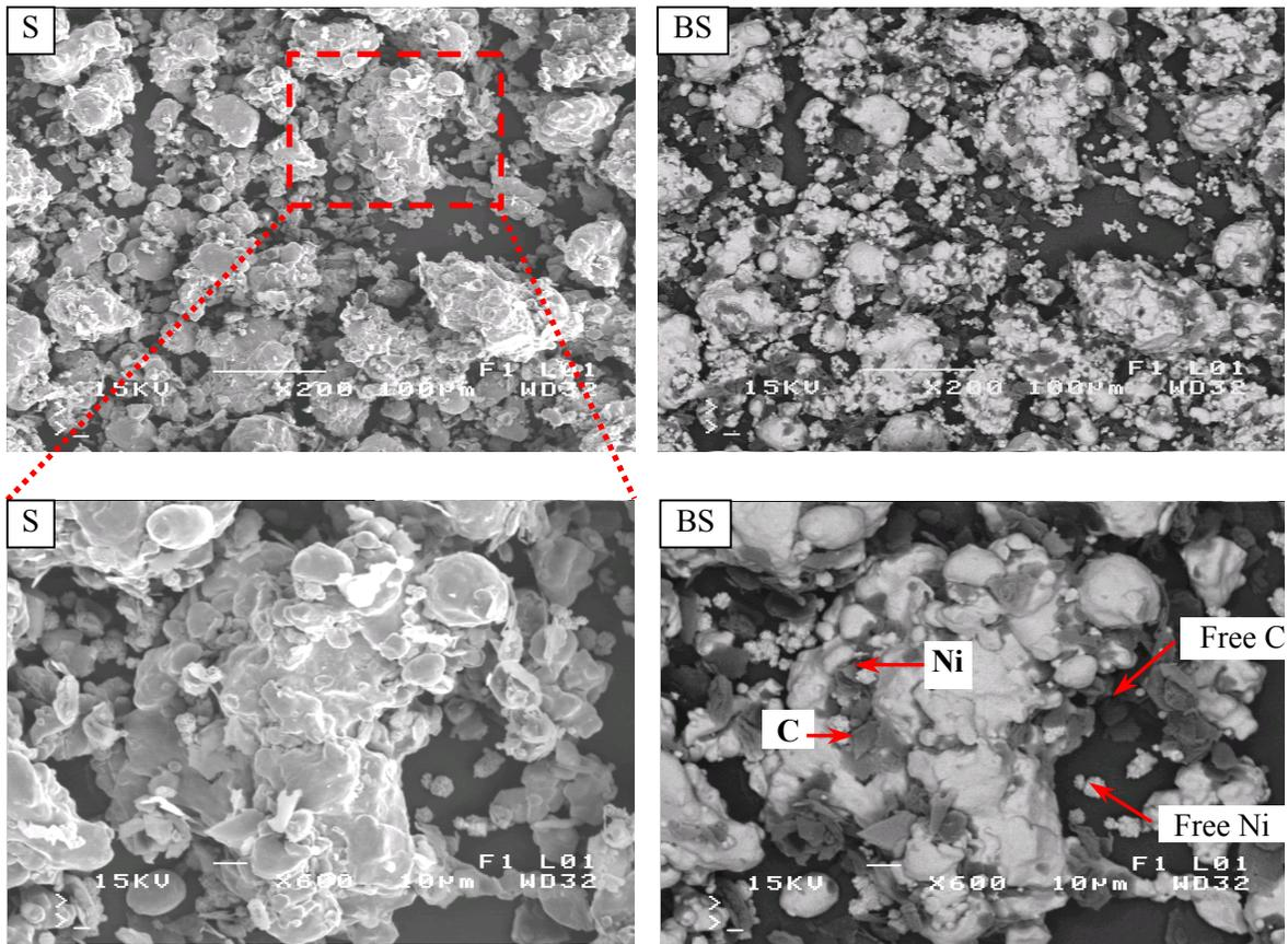
**Figure 2.** SEM micrographs of particles from a regular pre-mix made of ATOMET 1001, 2% Ni, 0.85% graphite and 0.75% wax. C represents either graphite or lubricant.
