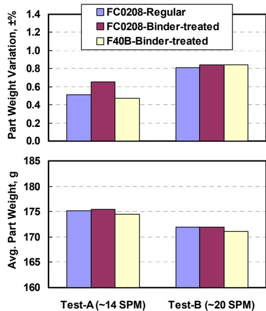
**Figure 10.** Results of test #1 carried out under easy filling conditions (Suction fill, fill height/wall thickness = 2).
