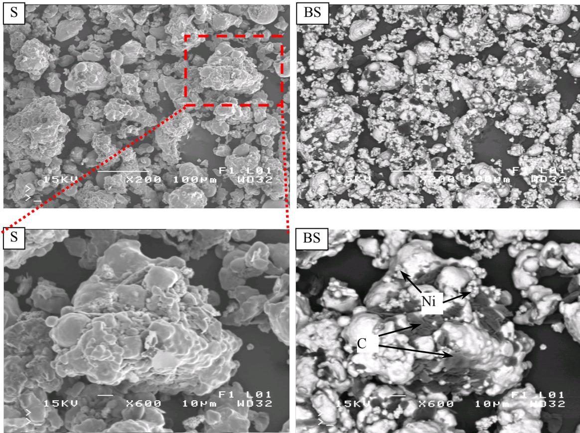
**Figure 3.** SEM micrographs of particles from a binder-treated mix made of ATOMET 1001, 2% Ni, 0.85% graphite and 0.75% wax+binder. C represents either graphite or lubricant. S is for secondary electron mode image and BS is for back-scattered electron mode image.
