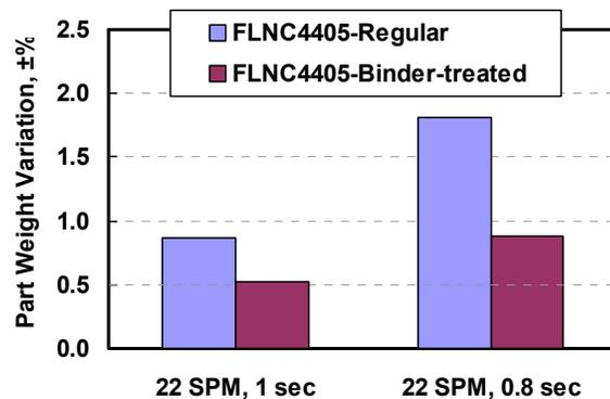
**Figure 11.** Variation in part weight obtained during test #2 carried out in *suction fill mode* under more difficult filling conditions (fill height/wall thickness = 8.2).
