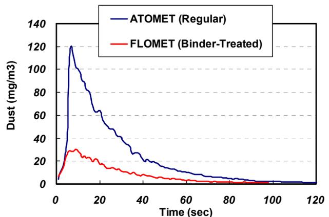
**Figure 7.** Quantity of dust (particles <math>< 10 \mu\text{m}</math>) created by a regular and a binder-treated F0008 mixes.
