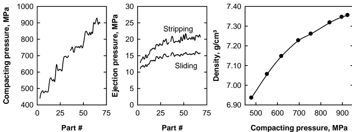
**Figure 9.** Increasing step-by-step compacting pressure (left), corresponding stripping and sliding ejection pressures (middle) and compressibility curve (right) for ATOMET EM-1 pressed into 16.5 mm thick gears using a composite lubricant in the die wall lubrication system.
