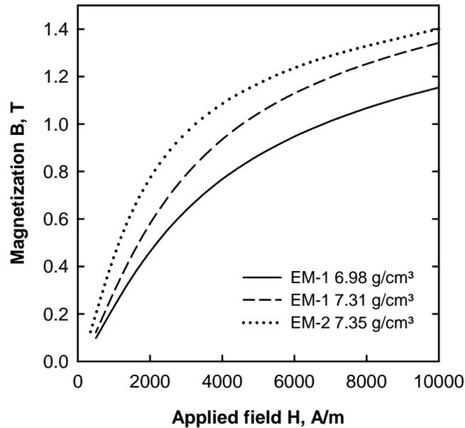
**Figure 6.** Typical magnetization curves of three different materials: iron-resin EM-1 at 6.98 g/cm<sup>3</sup> and 7.31 g/cm<sup>3</sup> density and iron-dielectric EM-2 at 7.35 g/cm<sup>3</sup> density.
