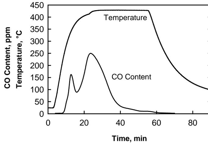
**Figure 11.** Temperature profile in a sample of ATOMET EM-2 and CO content read at the exit of a tubular furnace at 430°C as a function of time (375 g of parts, air flow of 2 l/min).
