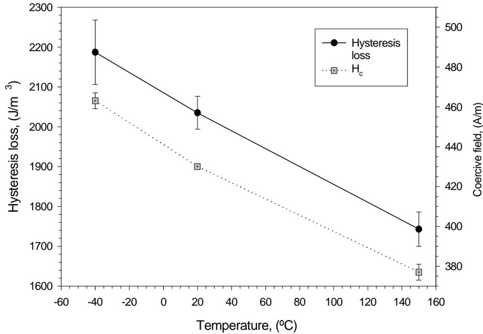
Figure 5. Variations of the hysteresis loss and coercive field with the temperature (-40°C, 20°C and 150°C) for iron-0.8% resin composite rings pressed at 65°C/620 MPa and cured at 175°C/1 h in air.
