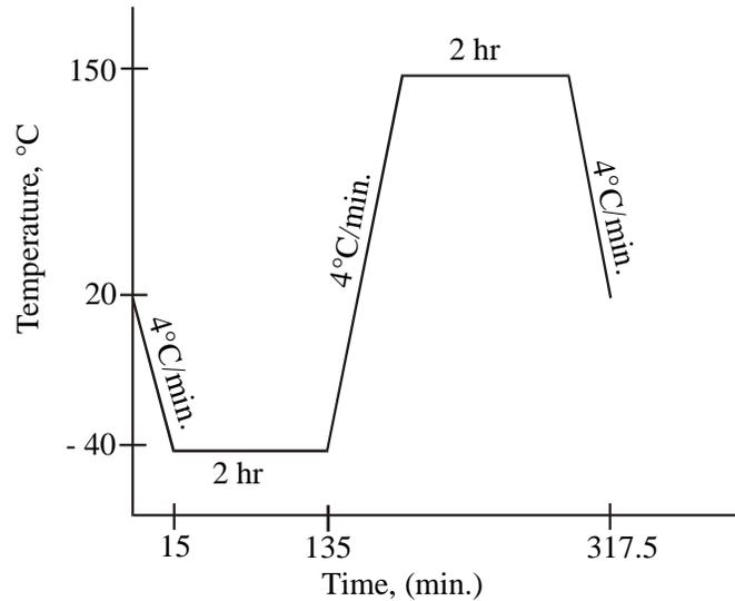
Figure 3: Thermal cycle profile used to simulate a thermal shock (according to SAE J1211 Standard).
