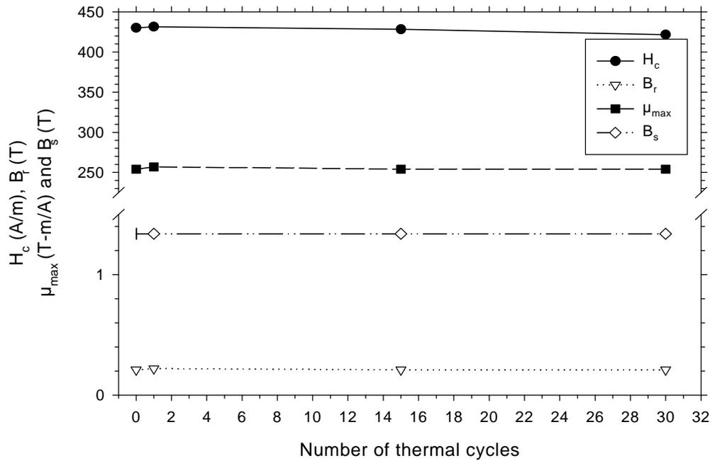
Figure 8: Effect of the number of thermal cycles (0, 1, 15 and 30) on DC magnetic properties of iron-0.8 % resin composites pressed at 65°C/620 MPa and cured at 175°C/1 h in air.
