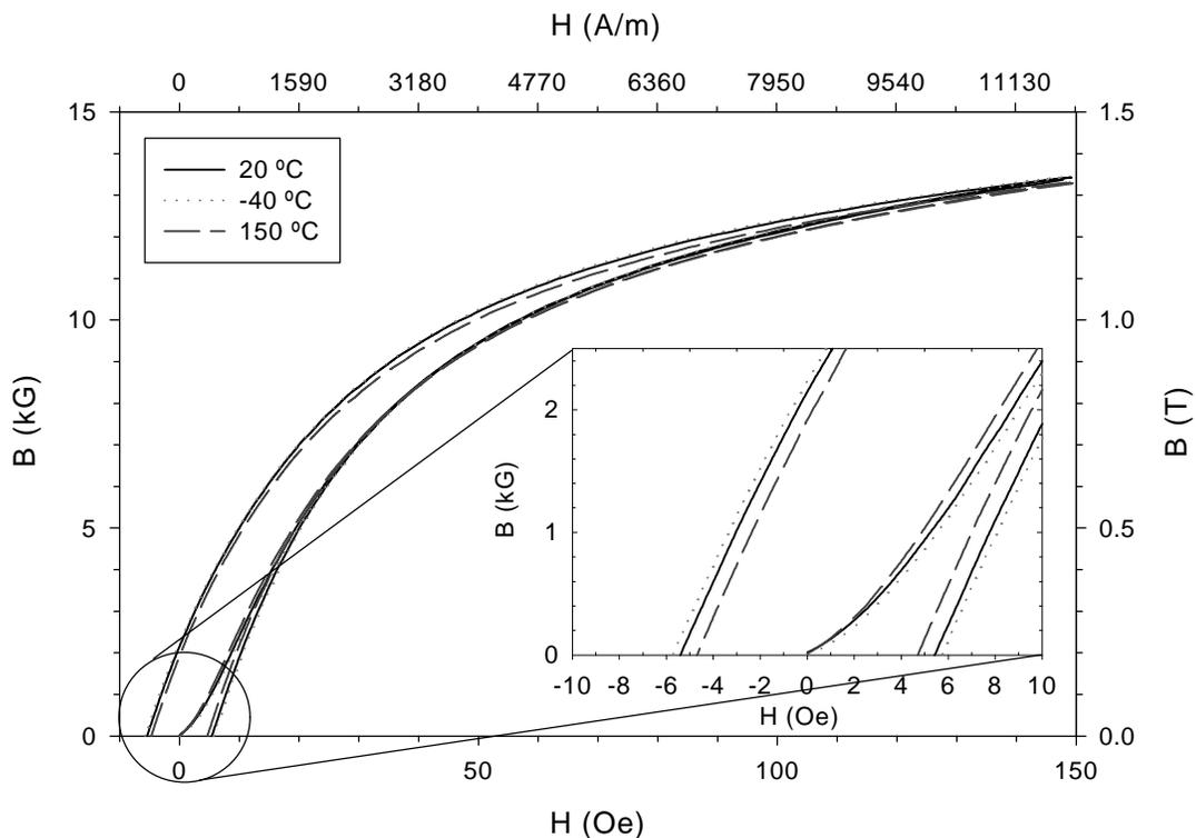
Figure 4. First half of the DC hysteresis loop of iron-0.8% resin composites at -40°C, 20°C and 150°C (rings pressed at 65°C/620 MPa and cured at 175°C/1 h in air).
