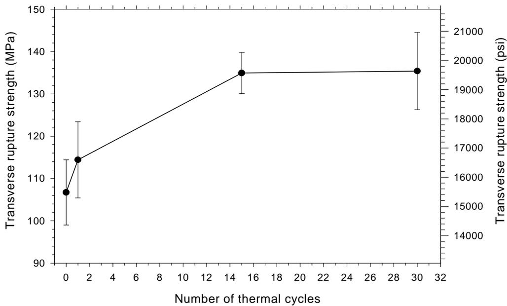
Figure 7: Effect of the number of thermal cycles on the transverse rupture strength of iron-0.8% resin composites pressed at 65°C/620 MPa and cured at 175°C/1 h in air. (Measured at 20°C on 5 bars per data point)
