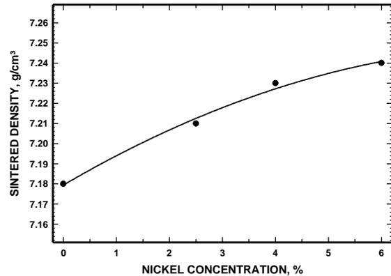
Figure 7. Effect of nickel concentration on the sintered density of TRS specimens pressed at 520 MPa and 130°C (ATOMET 4401+0.2% graphite+Ni+0.55% Lub; green density of 7.20 g/cm).
