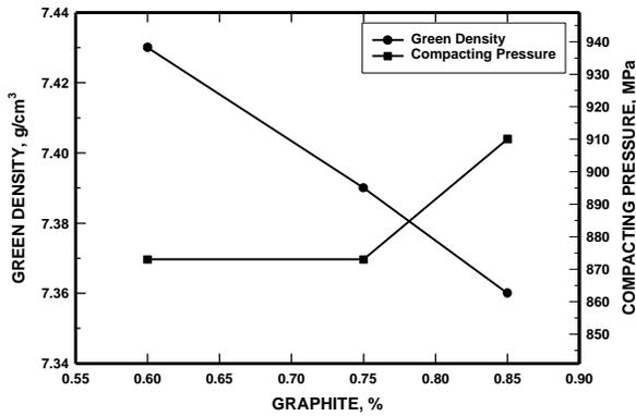
Figure 5. Effect of graphite concentration on the green density of TRS specimens pressed at 120°C (ATOMET 4401+4% Ni+1% Cu+ 0.5% lub).
