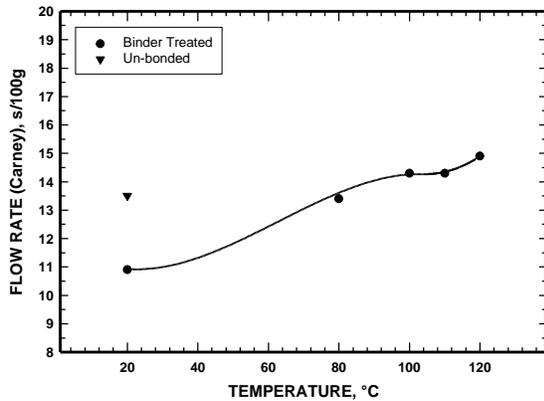
Figure 9. Effect of temperature on flowability of warm compaction mixes (ATOMET 1001+0.6% graphite+2% Ni+0.6% Lub).
