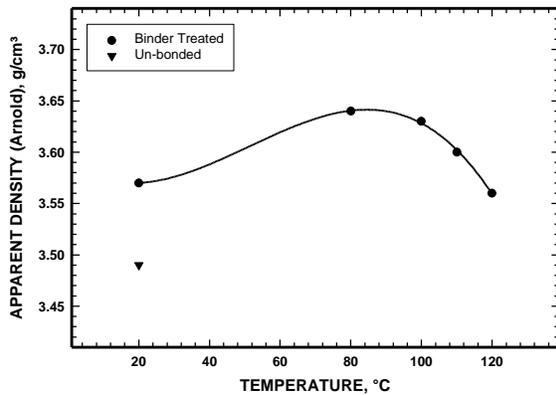
Figure 10. Effect of temperature on apparent density of warm compaction mixes (ATOMET 4401+4% Ni+1% Cu+0.85% graphite+0.6% Lub).
