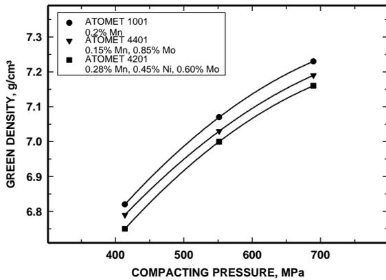
Figure 1. Compressibility of steel powders containing various concentrations of prealloyed elements (mixed with 0.5% lubricant pressed at room temperature), ref. 1.
