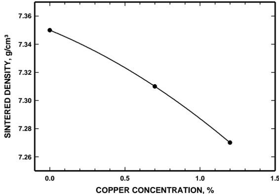
Figure 6. Effect of copper concentration on the sintered density of TRS specimens pressed at 130°C and 625 MPa (ATOMET 4401+3.5% Ni+0.3% graphite+Cu+0.5% lub; green density of 7.35 g/cm³).
