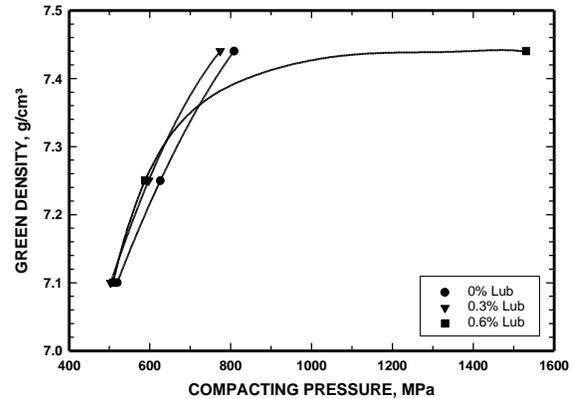
Figure 4. Effect of lubricant concentration on green density achieved during warm compaction (ATOMET 4401+0.6% graphite+4% Ni+lub; pressed at 150°C).
