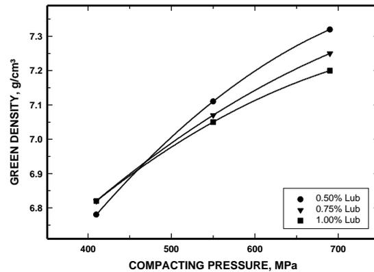
Figure 3. Effect of lubricant concentration and compacting pressure on the green density achieved after compaction (ATOMET 1001HP+zinc stearate, ref. 3).
