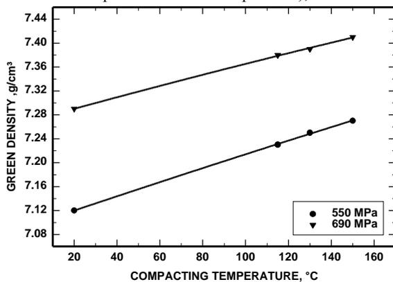
Figure 2. Effect of compacting temperature and pressure on green density (specimens pressed from ATOMET 1001 with 0.6% graphite and 2% Ni; die wall lubrication).
