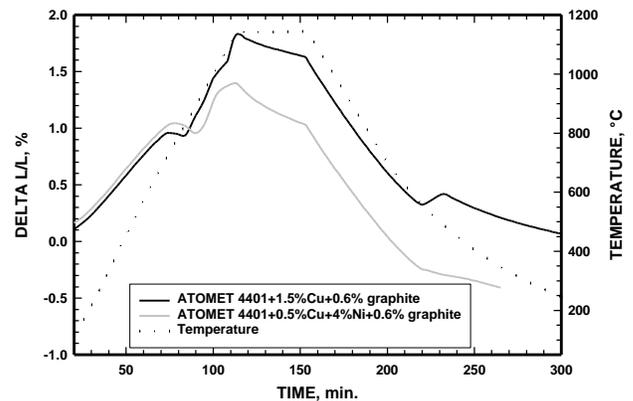
Figure 8. Effect of copper and nickel concentrations on dilatometric profiles of specimens sintered at 1145°C.
